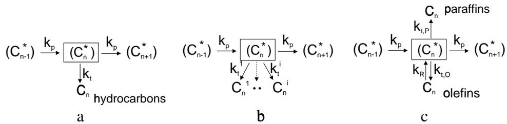
**Figure 2.15** Reaction growth schemes Fischer-Tropsch synthesis from Glebov and Kliger [97]. a. Classical Anderson-Schulz-Flory model with one termination constant for all products. b. Multiple termination probabilities originating from a single intermediate. c. Termination to paraffins and olefins, whereas the latter can be re-adsorbed on the catalytic surface.
