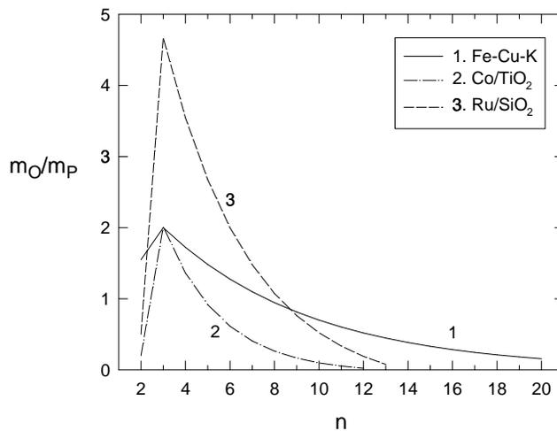
**Figure 2.8** Olefin to paraffin ratio on Co/TiO<sub>2</sub> ( $T=473$  K,  $H_2/CO=2.1$ ,  $P=2.0$  MPa, data from Iglesia et al. [89]), Ru/SiO<sub>2</sub> ( $T=485$  K,  $P=0.51$  MPa,  $H_2/CO=2$ , data from Madon et al. [32]), and precipitated Fe/Cu/K ( $T=489$  K,  $P=1.62$  MPa,  $H_2/CO=2$ , data from Madon et al. [32])
