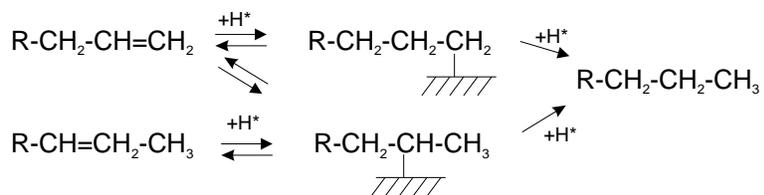
**Figure 2.4** Secondary reactions of olefins (Schulz et al. [74]).
