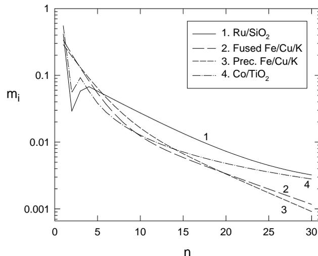
**Figure 2.7** Total hydrocarbon selectivity on Co/TiO<sub>2</sub> ( $T=473$  K,  $H_2/CO=2.1$ ,  $P=2.0$  MPa, data from Iglesia et al. [89]), Ru/SiO<sub>2</sub> ( $T=485$  K,  $H_2/CO=2$ ,  $P=0.51$  MPa, data from Madon et al. [32]), and fused and precipitated Fe/Cu/K (data from Donnelly et al. [88]).
