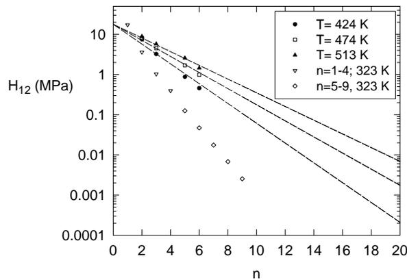
**Figure 2.20** Henry's constants of n-paraffins in eicosane at  $T=323\text{K}$  (Chappelow and Prausnitz [130] and Donohue et al. [131]) and in octacosane at  $T=424, 474,$  and  $513\text{K}$  (Breman et al. [129]), dotted lines are calculated with the vapor pressure correlation for  $\text{C}_9\text{-C}_{29}$  (Caldwell and van Vuuren [132]).
