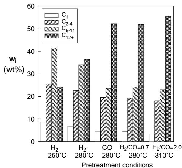
**Figure 2.11** Effect of pretreatment conditions on the hydrocarbon selectivity at 250 °C, 1.48 MPa,  $H_2/CO = 0.67$ ,  $5.5 \cdot 10^{-4} \text{ Nm}^3 \text{ kg}_{cat}^{-1} \text{ s}^{-1}$  from Bukur et al. [38].
