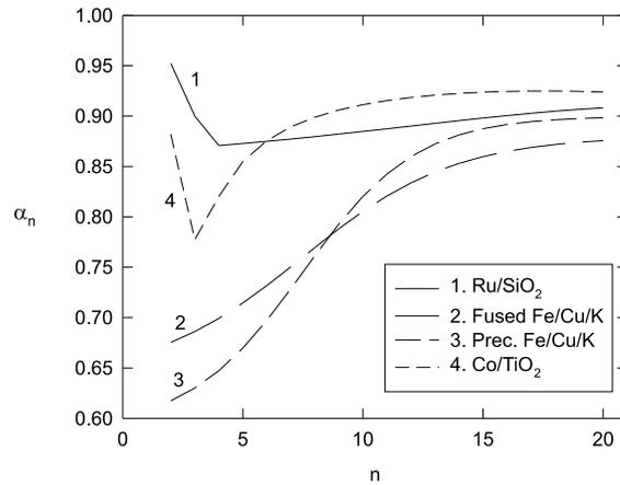
**Figure 2.17** Chain growth probability factor ( $\alpha_n$ ) as function of chain length  $n$ , data from Madon et al. [32] (Ru/SiO<sub>2</sub>, and Co/TiO<sub>2</sub>) and Donnelly et al. [88] (fused and precipitated Fe/Cu/K).
