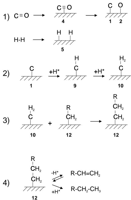
**Figure 2.3** Carbide mechanism for the Fischer-Tropsch synthesis [18, 73].
