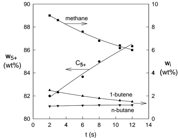
**Figure 2.10** Residence time effect on methane, C<sub>5+</sub>, n-butane, and 1-butene selectivity on Co/TiO<sub>2</sub> (473 K, 2.0 MPa, H<sub>2</sub>/CO= 2.1, 9.5-72 % CO conversion [3]).
