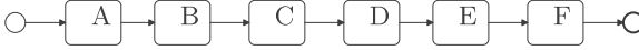
Fig. 2. Sample process model ( X\#duration \sim N(500, 50) \forall X \in \{A, \dots, F\} )
