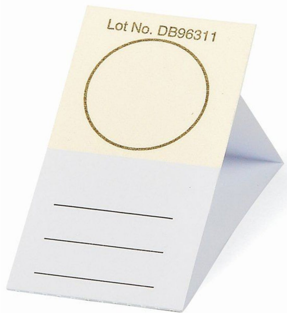
Fig. 2 A Whatman FTA micro card. The sampling area is within the circle. Image taken from Fisher Scientific
