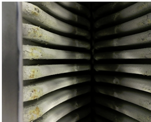
Fig. 9. Silica deposition in the aluminium finned heat exchanger of appliance 4 roughly 950 h of operation using 11.2 \text{ mg Si/m}^3 .
