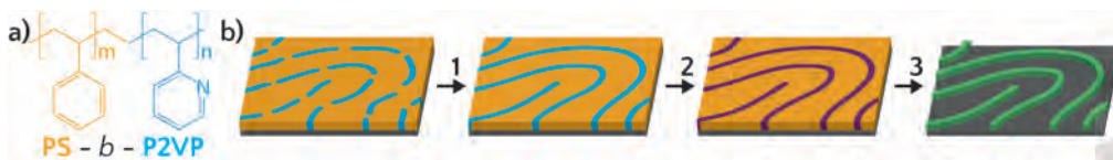
Figure 2.2 | a) Chemical structure of PS- b -P2VP and b) a schematic overview of the sample fabrication steps for polymer templating. The BCP film is spin coated on a silicon wafer and undergoes self-assembly during the solvent vapor annealing (SVA) step in chloroform (1). In order to allow for the inclusion of the metal oxide precursor solution, the sample undergoes a second SVA step in ethanol to swell and allow for metal ion inclusion into the P2VP block by spin coating (2). Subsequent UV-ozone treatment and thermal annealing results in the oxidation of the metal oxide precursor and the removal of the polymer matrix, leaving a metal oxide nanostructure (3).
