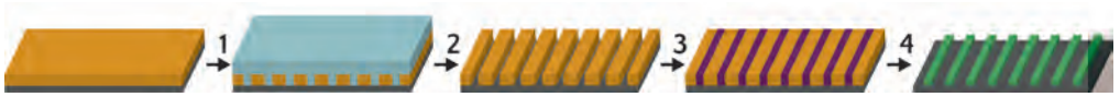
Figure 2.1 | Schematic overview of the sample fabrication steps in polymer imprinting. A PS film is spin coated on a silicon wafer and a PDMS stamp is applied to the film (1) under a load of 200 g at a temperature of 150 °C. Once the imprinting is finished, and the sample has cooled down to well below the glass transition temperature of PS, the PDMS stamp is removed and the PS film shows the imprinted structure (2). Using spin coating, the metal oxide precursor solution is loaded into the imprinted film (3) and subsequent thermal annealing results in the oxidation of the metal oxide precursor and the removal of the polymer matrix, leaving a metal oxide nanostructure (4).
