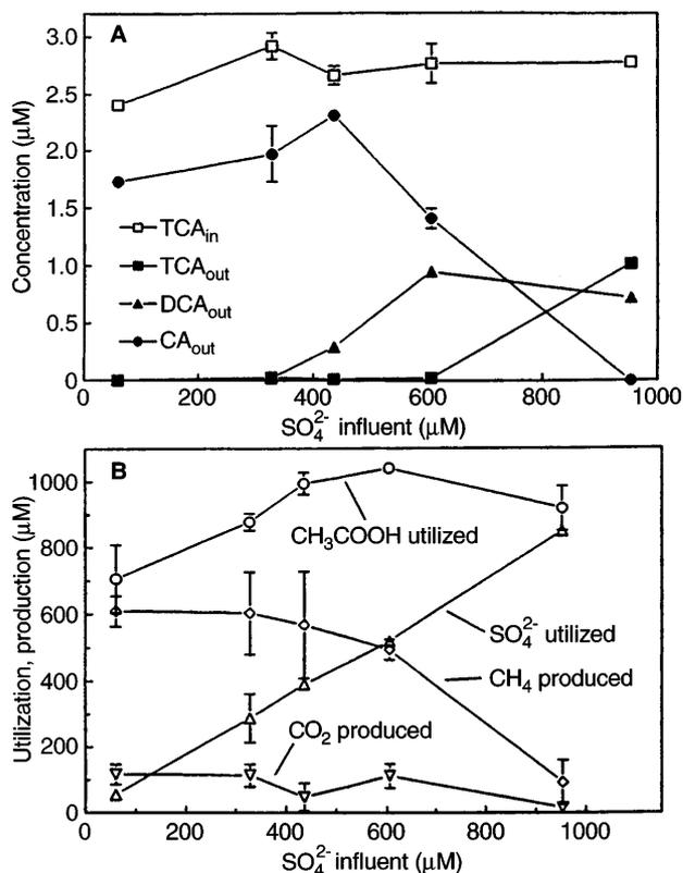
**Fig. 3** Effect of sulfate concentration on the transformation of 1,1,1-trichloroethane (TCA) (A) and acetate conversion (B) in an anaerobic packed-bed reactor. Error bars standard deviations on two to five measurements taken within 7 days
