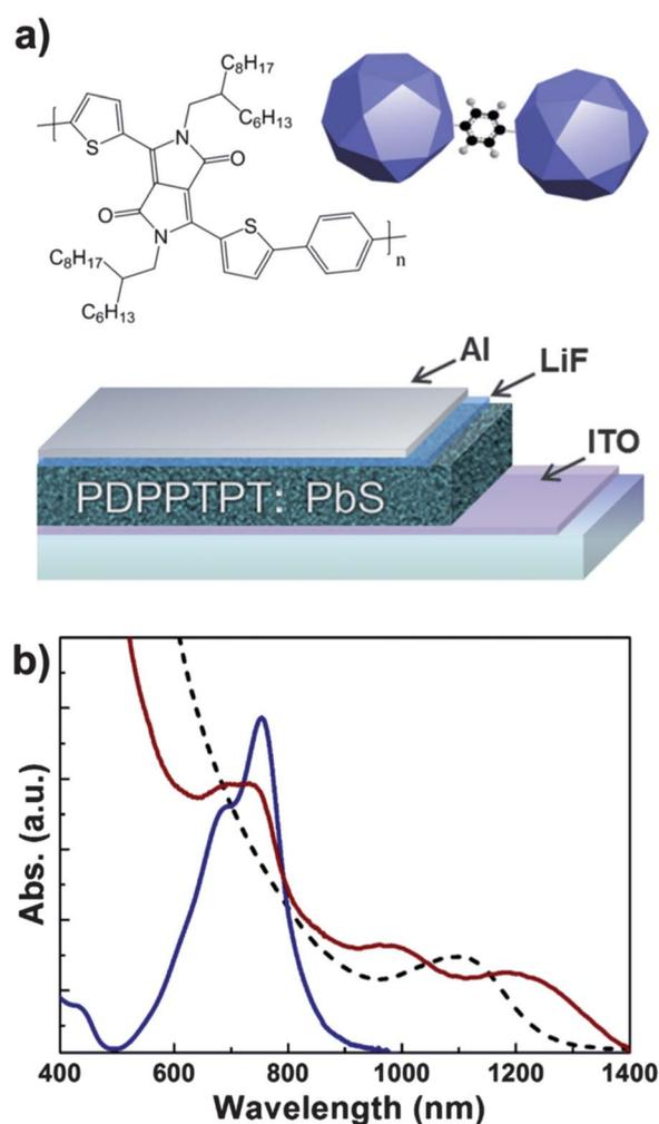
**Fig. 1** (a) Molecular structure of the PDPPTPT polymer, schematic of the BDT crosslinked PbS nanocrystals and of the device structure. (b) Absorption spectra of the PDPPTPT film (blue line), OA-capped PbS nanocrystals dispersed in toluene (dashed black line) and of the PDPPTPT:PbS (10 : 90 wt%) blend film (red line) after the BDT ligand exchange treatment.
