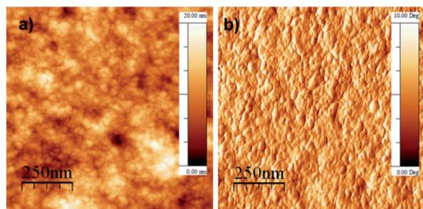
**Fig. 2** Atomic force microscopy images in tapping mode: (a) surface morphology and (b) phase of the PDPPTPT:PbS (10 : 90 wt%) blend after the BDT treatment, the scan area is  $1 \times 1 \mu\text{m}$ , RMS roughness 2.7 nm.
