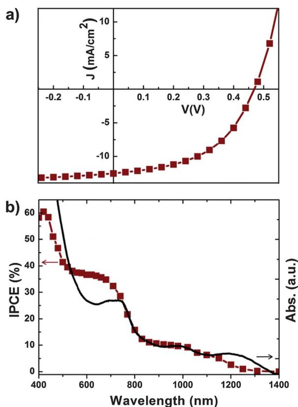
**Fig. 3** (a)  $J$ - $V$  characteristic of the PDPPTPT:PbS (10 : 90 wt%) blend device under AM 1.5G ( $100 \text{ mW cm}^{-2}$ ) illumination. (b) Plots of the IPCE of the blend device (red square) and the absorption spectrum (black line) of the BDT-treated blend film.
