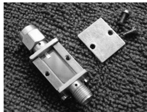
FIG. 2. Photo of a home-built heat-sink for use in cryogenic coaxial lines, with SMA connectors and a gold-plated sapphire substrate in a copper housing unit.
