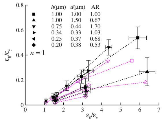
FIG. 8. (Color online)  $\varepsilon_B$  as a function of  $\varepsilon_0$  predicted for columnar-grained films by the constrained model after a refit of the source density, see Fig. 7. The corresponding unconstrained results (open symbols) are superimposed from Fig. 4.
