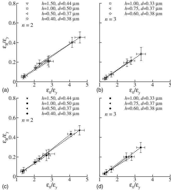
FIG. 9.  $\epsilon_B$  as a function of  $\epsilon_0$  for multilayer films unloaded from  $\epsilon_0 = 0.005$  and  $0.01$ . (a) and (b) Unconstrained model, and (c) and (d) Constrained model. Dashed lines are drawn as a guide to the eye.
