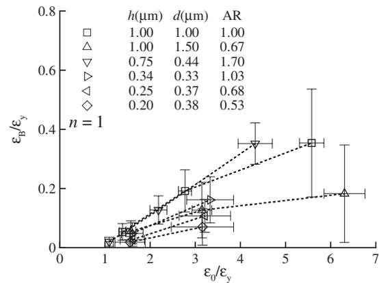
FIG. 4.  $\varepsilon_B$  as a function of prestrain  $\varepsilon_0$ , both normalized by the yield strain as defined in the inset of Fig. 3, for columnar-grained films unloaded from  $\varepsilon_0 = 0.005$  and  $0.01$ . Films with thickness 1 and 0.75  $\mu\text{m}$  have been unloaded from  $\varepsilon_0 = 0.0025$ . Dashed lines are drawn as a guide to the eye.
