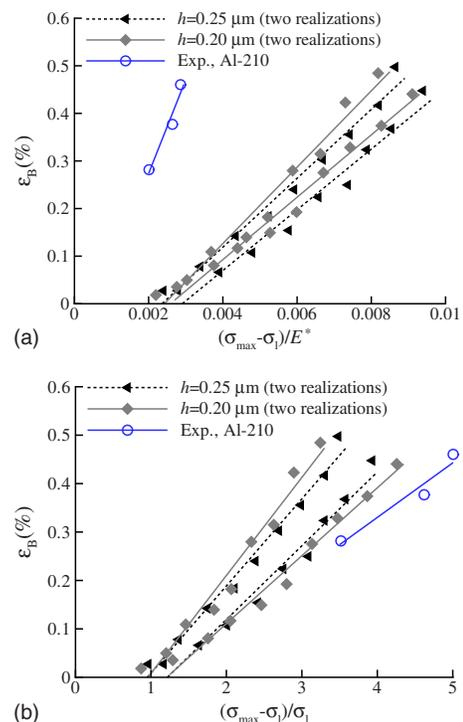
FIG. 14. (Color online) (a)  $\varepsilon_B$  vs  $(\sigma_{\max} - \sigma_1)/E^*$  and (b)  $\varepsilon_B$  vs  $(\sigma_{\max} - \sigma_1)/\sigma_1$ . For comparison purpose, experimental data that has a similar polydispersity of grain size is also shown. The experimental data is from Ref. 2.
