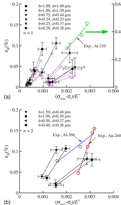
FIG. 12. (Color online)  $\epsilon_B$  as a function of  $(\sigma_{max} - \sigma_1)/E^*$  by using the constrained model. In (a), the results after refitting are shown together with the corresponding unconstrained results (open symbols). The experimental data are from Ref. 2. Dashed lines are drawn as a guide to the eye.
