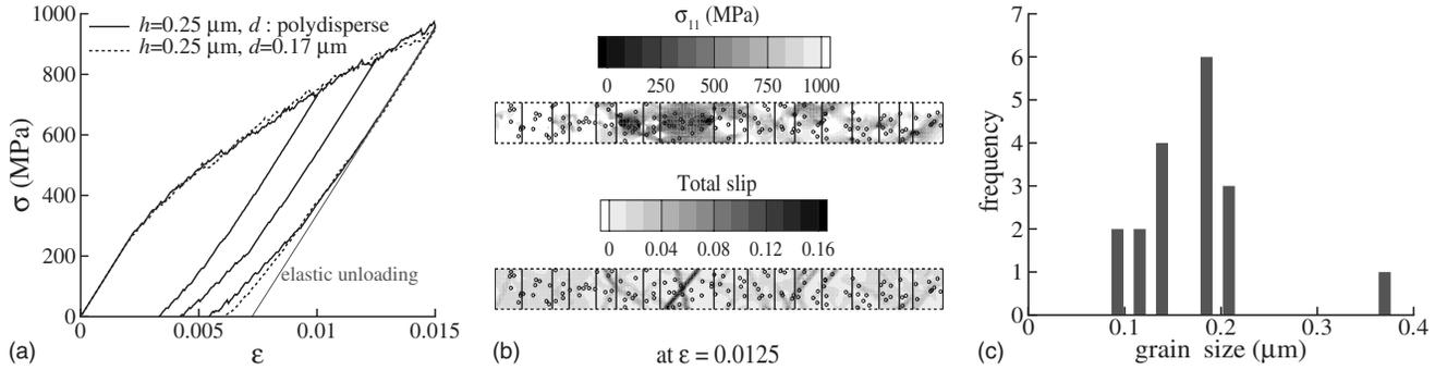
FIG. 13. (a) Stress-strain response of 0.25  $\mu\text{m}$  thick film with columnar grains having different sizes. (b) Distribution of the tensile direction stress and the total slip at  $\varepsilon=0.0125$ , with the sources (circles) superimposed. (c) Grain size distribution in the computational cell, corresponding to an average of 0.17  $\mu\text{m}$ . The response for this average grain size is shown in (a) with a dashed line, for comparison.
