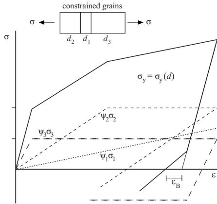
FIG. 15. Qualitative response of a constrained film model comprising three grains, with sizes  $d_1 < d_2 < d_3$ , each exhibiting size-dependent, perfect plasticity. The dashed lines represent the response of individual grains, multiplied by their respective volume fraction  $\psi$ . The overall response, shown as the solid curve, reveals a BE upon unloading as indicated.
