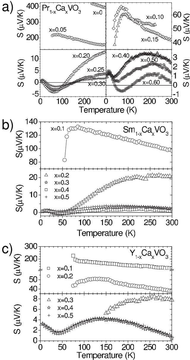
FIG. 3. Temperature dependence of the Seebeck coefficient in (a)  $\text{Pr}_{1-x}\text{Ca}_x\text{VO}_3$ , (b)  $\text{Sm}_{1-x}\text{Ca}_x\text{VO}_3$ , and (c)  $\text{Y}_{1-x}\text{Ca}_x\text{VO}_3$ .
