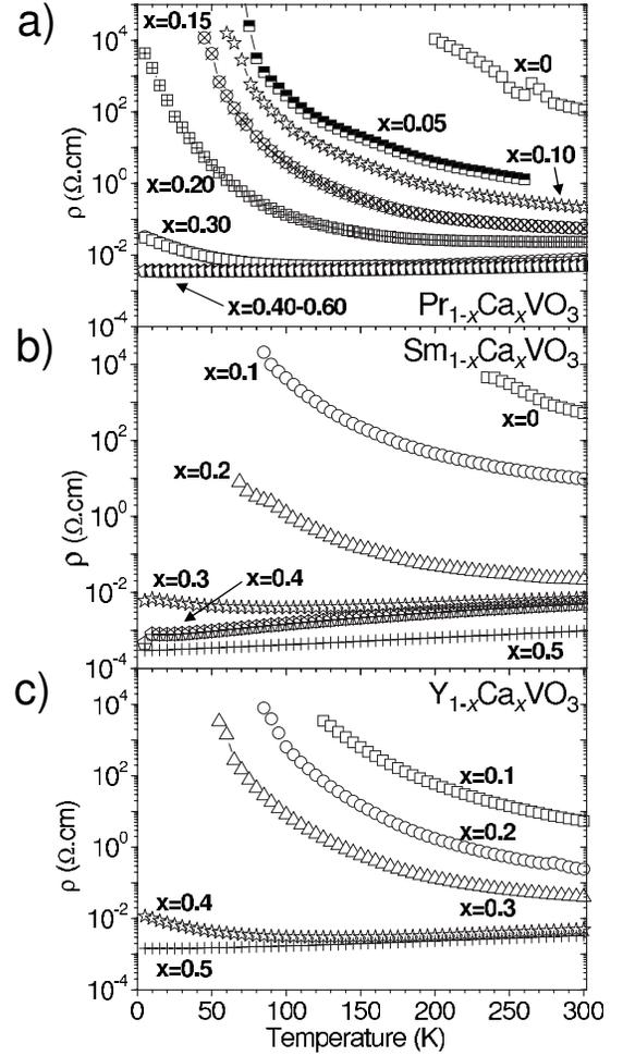
FIG. 1. Temperature dependence of the resistivity of (a)  $\text{Pr}_{1-x}\text{Ca}_x\text{VO}_3$ , (b)  $\text{Sm}_{1-x}\text{Ca}_x\text{VO}_3$ , and (c)  $\text{Y}_{1-x}\text{Ca}_x\text{VO}_3$ . Note that  $\rho$  is plotted on a logarithmic scale.
