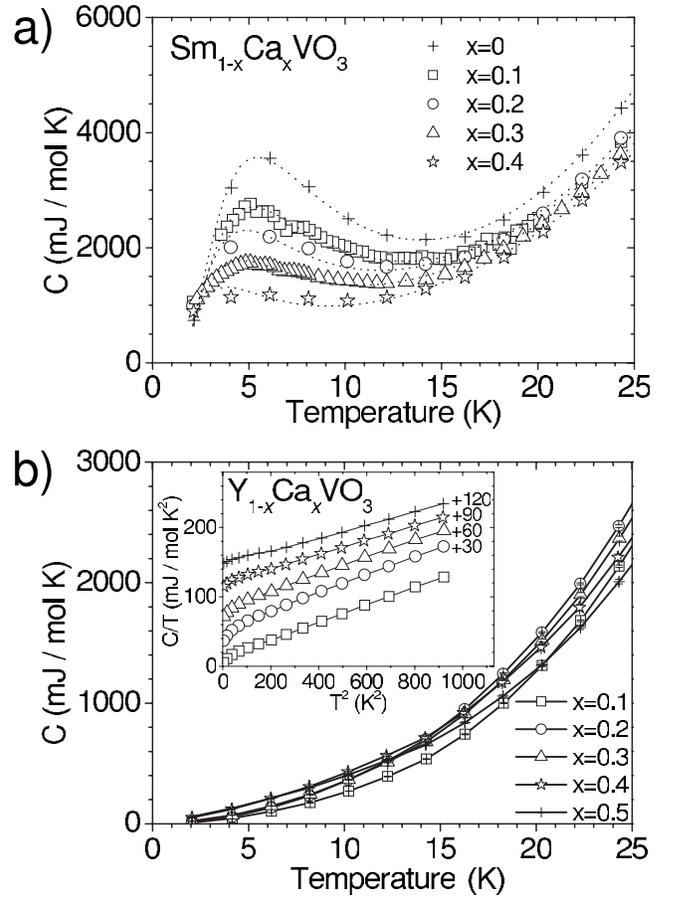
FIG. 4. Evolution of the low-temperature specific heat of (a)  $\text{Sm}_{1-x}\text{Ca}_x\text{VO}_3$  and (b)  $\text{Y}_{1-x}\text{Ca}_x\text{VO}_3$ . The dotted lines in (a) are fits to the Schottky anomaly by using Eq. (8). The inset of (b) shows plots of  $C/T$  versus  $T^2$ , in which, for reasons of clarity, the data for  $x \geq 0.2$  have been offset by the factors indicated.
