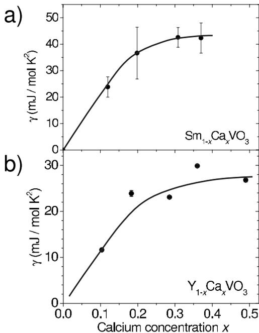
FIG. 5. Evolution of the electronic term of the specific heat,  $\gamma$ , with  $x$  for (a)  $\text{Sm}_{1-x}\text{Ca}_x\text{VO}_3$  and (b)  $\text{Y}_{1-x}\text{Ca}_x\text{VO}_3$ . The solid lines are guides for the eye.
