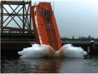
Fig. 1 Drop test with free-fall lifeboat (from: www.verhoef.eu)
