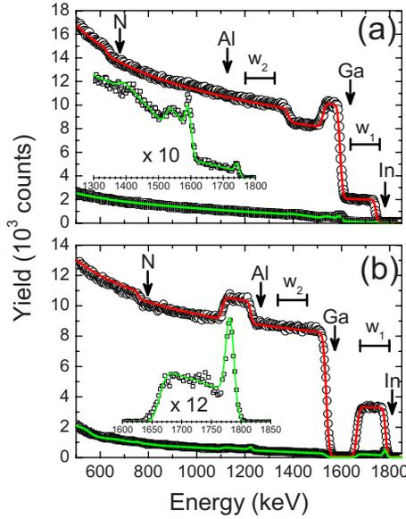
FIG. 1. (Color online) Random and  $\langle 0001 \rangle$  aligned spectra (circles and squares) and simulation (solid line) from RBS/C experiments at 2 MeV. The insets show the aligned spectrum in detail. Windows of the film ( $w_1$ ) and the substrate ( $w_2$ ) signals for the angular scans are also shown.
