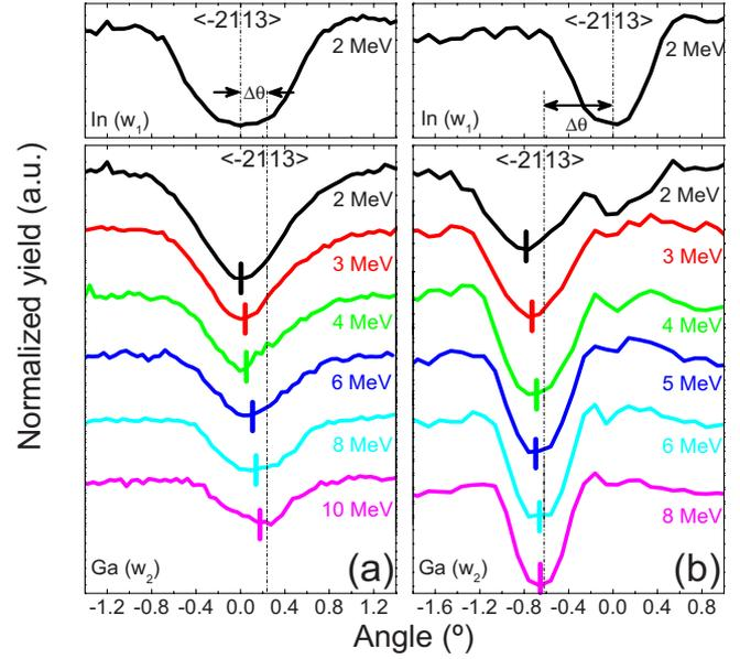
FIG. 2. (Color online) Experimental angular scans across the  $\langle \bar{2}113 \rangle$  axis for different energies in strained AlGaInN/GaN (a) and AlInN/GaN (b) HSS. As a reference, the angular scan from the active layer ( $w_1$ ) at 2 MeV is shown (top graphics). The horizontal lines mark the value of the real kink angle for both HSS. The shift from the substrate ( $w_2$ ) does not match  $\Delta\theta$  due to steering effects, which gradually diminish with energy.
