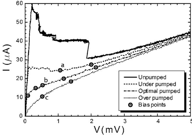
FIG. 2. Unpumped, underpumped, optimal pumped, and over pumped  $I/V$  curves. Circles indicate the bias points where reflection and mixer gain measurements were obtained. a, b, and c refer to the impedances shown in Fig. 3.
