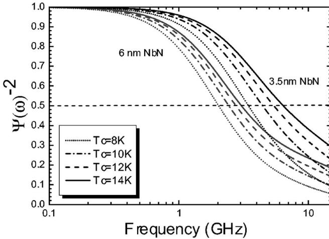
FIG. 6.  $\Psi(\omega)^{-2}$  as a function of IF frequency for 3.5 and 6 nm thickness NbN films of different  $T_c$ .  $\Psi(\omega)^{-2}$  can be interpreted as the relative conversion gain without the effect of electrothermal feedback. For an optimized NbN mixer the maximum gain bandwidth is projected to be on the order of 5.5–6 GHz.
