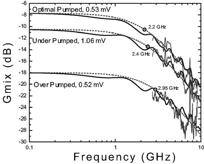
FIG. 4. Measured and modeled HEB mixer conversion gain as a function of IF frequency for the three bias conditions in Fig. 3. The  $-3$  dB gain rolloff shifts to higher frequency with increased LO power. This is understood to be caused by the increased mean electron temperature. The effect of electro-thermal feedback is taken into account by means of the (modeled) complex IF load impedance. Details in Tables I and II.
