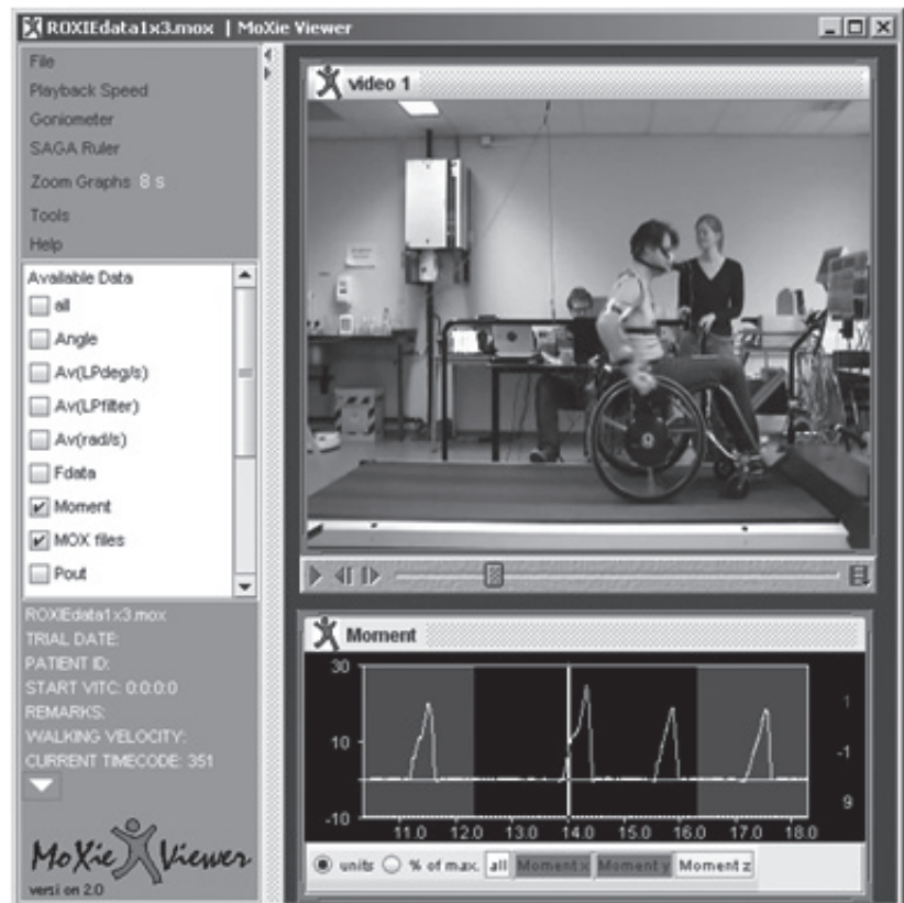
Fig. 6. MoXie Viewer (VU medical center, Amsterdam, The Netherlands): software for synchronously viewing video and concurrently acquired signals such as force and torque data.
