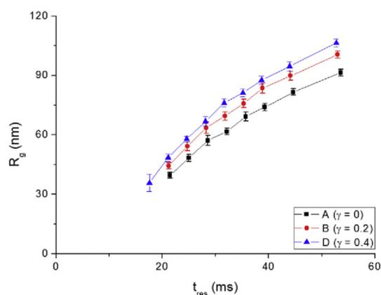
**Fig. 1 – Radius of gyration  $R_g$  as function of residence time  $t_{res}$  for stoichiometric flames A, B and D with hydrogen fuel fractions  $\gamma = 0, 0.2$  and 0.4.**
