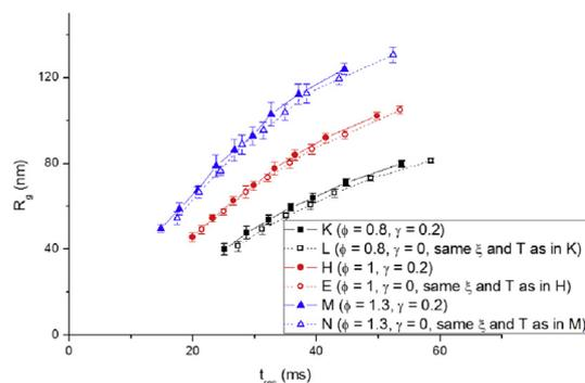
**Fig. 6** – Radius of gyration  $R_g$  as function of residence time  $t_{res}$  for hydrogen/methane/air flames with  $\gamma = 0.2$  and methane/air flames at  $\phi = 0.8$  (flames K and L),  $\phi = 1.0$  (flames E and H) and  $\phi = 1.3$  (flames M and N). The methane/air flames have the same temperature and concentration  $\xi$  of silica in the combustion products as the corresponding flames with added hydrogen of the same  $\phi$ .
