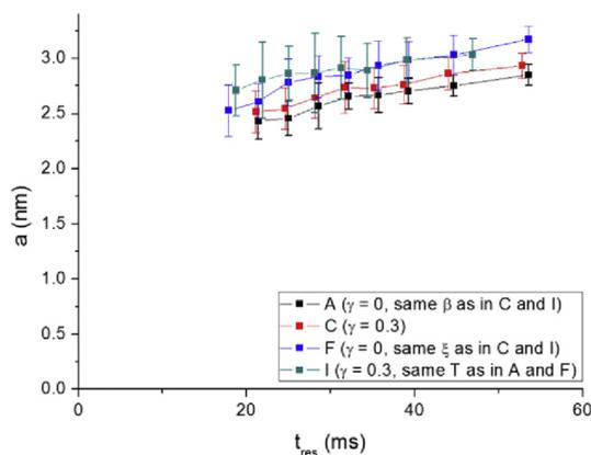
**Fig. 5** – Monomer radius  $a$  as function of residence time  $t_{res}$  for stoichiometric flames: flames C and I with hydrogen fuel fraction  $\gamma = 0.3$  and two methane/air flames, one with the same concentration of L2 in fuel  $\beta$  (flame A) and another with the same concentration of silica in the combustion products  $\xi$  (flame F).
