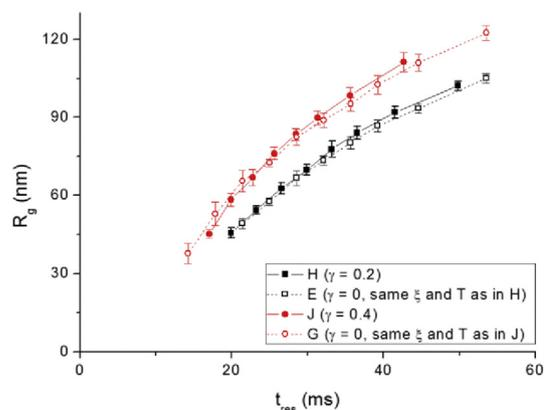
**Fig. 3** – Radius of gyration  $R_g$  for stoichiometric flames H and J with hydrogen fuel fractions of 0.2 and 0.4, respectively, and corresponding reference flames E and G with equal concentration of silica in the combustion products  $\xi$ , all at  $T = 1855$  K.
