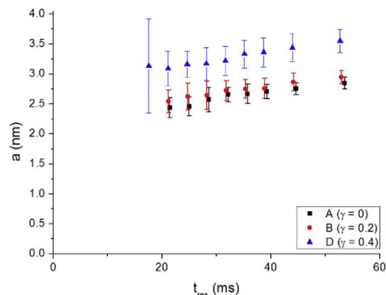
**Fig. 4** – Monomer radius  $a$  as function of residence time  $t_{\text{res}}$  for stoichiometric flames A, B and D with hydrogen fuel fractions  $\gamma = 0, 0.2$  and  $0.4$ .
