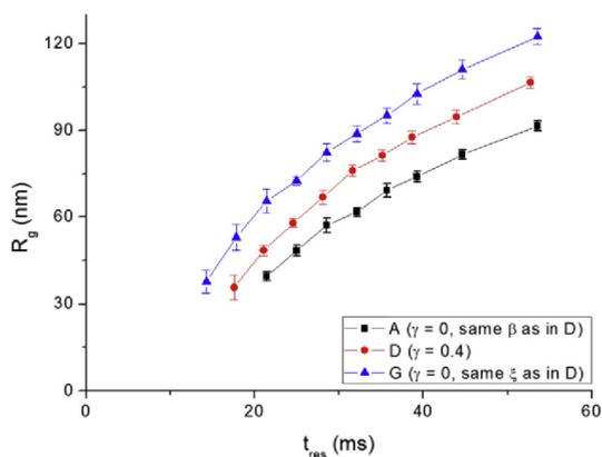
**Fig. 2** – Radius of gyration  $R_g$  as function of residence time  $t_{\text{res}}$  for stoichiometric flames: flame D with hydrogen fuel fraction  $\gamma = 0.4$  and two methane/air flames, one with the same concentration of L2 in fuel  $\beta$  (flame A) and the other with the same concentration of silica in the combustion products  $\xi$  (flame G).
