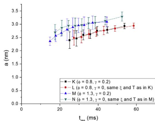
**Fig. 7** – Comparison of monomer radius  $a$  as function of residence time  $t_{res}$  for lean flames at  $\phi = 0.8$  with hydrogen fuel fraction  $\gamma = 0.2$  (flame K) and pure methane/air flame with equal concentration of silica in the combustion products  $\xi$  and flame temperature (flame L), and rich flames at  $\phi = 1.3$  with  $\gamma = 0.2$  (flame M) and pure methane/air flame with equal  $\xi$  and flame temperature (flame N).
