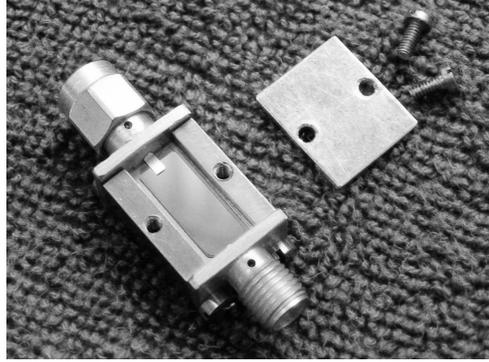
**Figure 5.2:** Photo of a home-built heat-sink for use in cryogenic coaxial lines, with SMA connectors and a gold-plated sapphire substrate in a copper housing unit.
