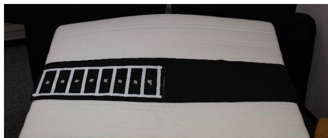
Figure 4. ISABel II, a 160 \times 200 cm double bed with two sensor mattresses giving a total lateral resolution of 16 \times 1 sensor elements. Only the eight sensor elements in contact with the participant are used for the position classification.
