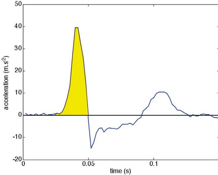
**Figure 5.6.** One of the two accelerometer signals in a strike on the punching bag. The impulses of the punch are equal to the shaded area under the curves times
