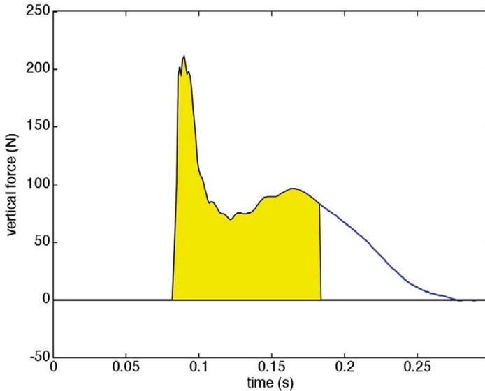
**Figure 5.5.** The low-pass filtered force signal of a stamp. The impulse of the foot
