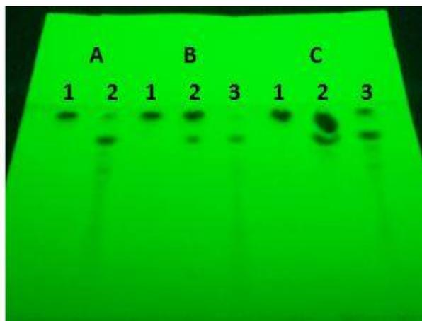
**Figure 1.** TLC analysis of ethyl gallate (EG) glycosylation by free Gtf180-ΔN (1000 mM sucrose, 4 U/mL enzyme), visualized by UV (254 nm). **A** 100 mM EG, 0% ethyl acetate; **B** 100 mM EG, 37.5% ethyl acetate; **C** 400 mM EG, 37.5% ethyl acetate. **A1, B1, C1** Incubation mixture without enzyme; **A2** 60 min incubation; **B2, C2** 60 min incubation (ethyl acetate phase); **B3, C3** 60 min incubation (aqueous phase).
