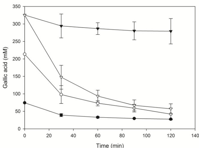
**Figure 2.** Depletion of gallic acid (GA) due to its glycosylation by free Gtf180-ΔN (1000 mM sucrose, 4 U/mL enzyme): ● 80 mM GA, 0% DMSO; ○ 210 mM GA, 10% DMSO; ▼ 325 mM GA, 20% DMSO; and by immobilized Gtf180-ΔN (1000 mM sucrose, 4 U/mL enzyme): ▽ 325 mM GA, 20% DMSO.
