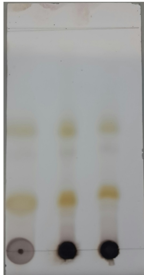
Fig. 5. TLC profile of ZO extract (left) and ODFs containing ZO (middle and right).
