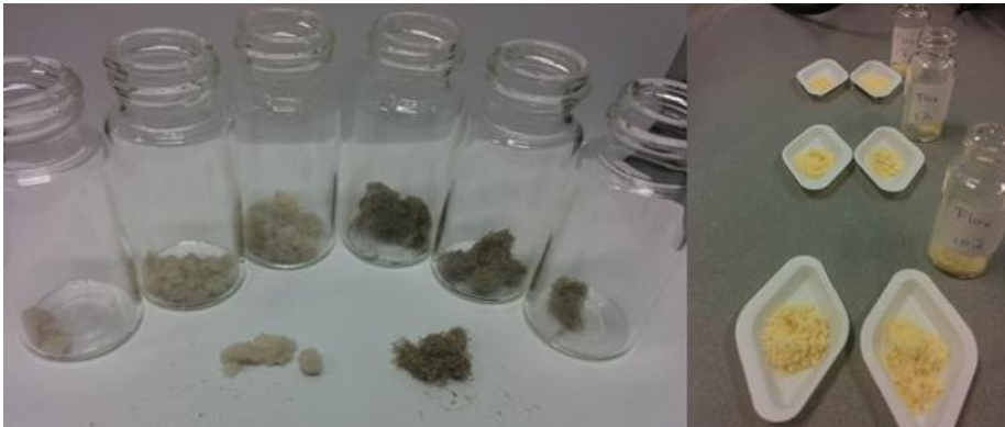
Figure 2: Flax (left) and Jute (right) fibers used and fiber/polymer (PE-fur) mixtures (far right)
