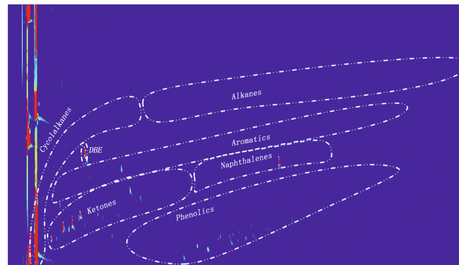
Figure S3-8. GCxGC chromatogram for a liquid product from an experiment with Pt/ZrO 2 (400 °C, 3 h).
