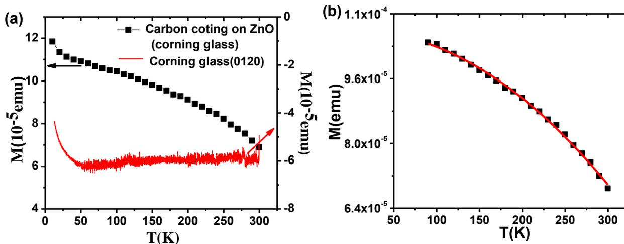
**Figure 3.5** (a) Temperature dependence of magnetization of a carbon-coated ZnO film and of the Corning glass substrate. The applied field was 1 T. (b) Bloch law fit to the  $M$ - $T$  data of (a),  $90 \text{ K} < T < 300 \text{ K}$ .
