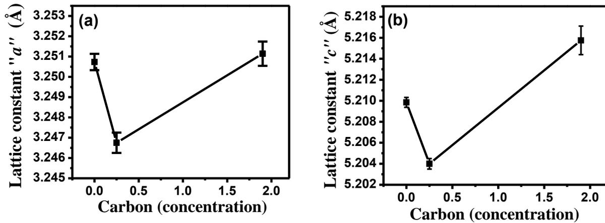
**Figure 3.2** Variation of lattice parameters (a) “a” and (b) “c” in carbon-doped ~300 nm thick ZnO films with different carbon concentration.
