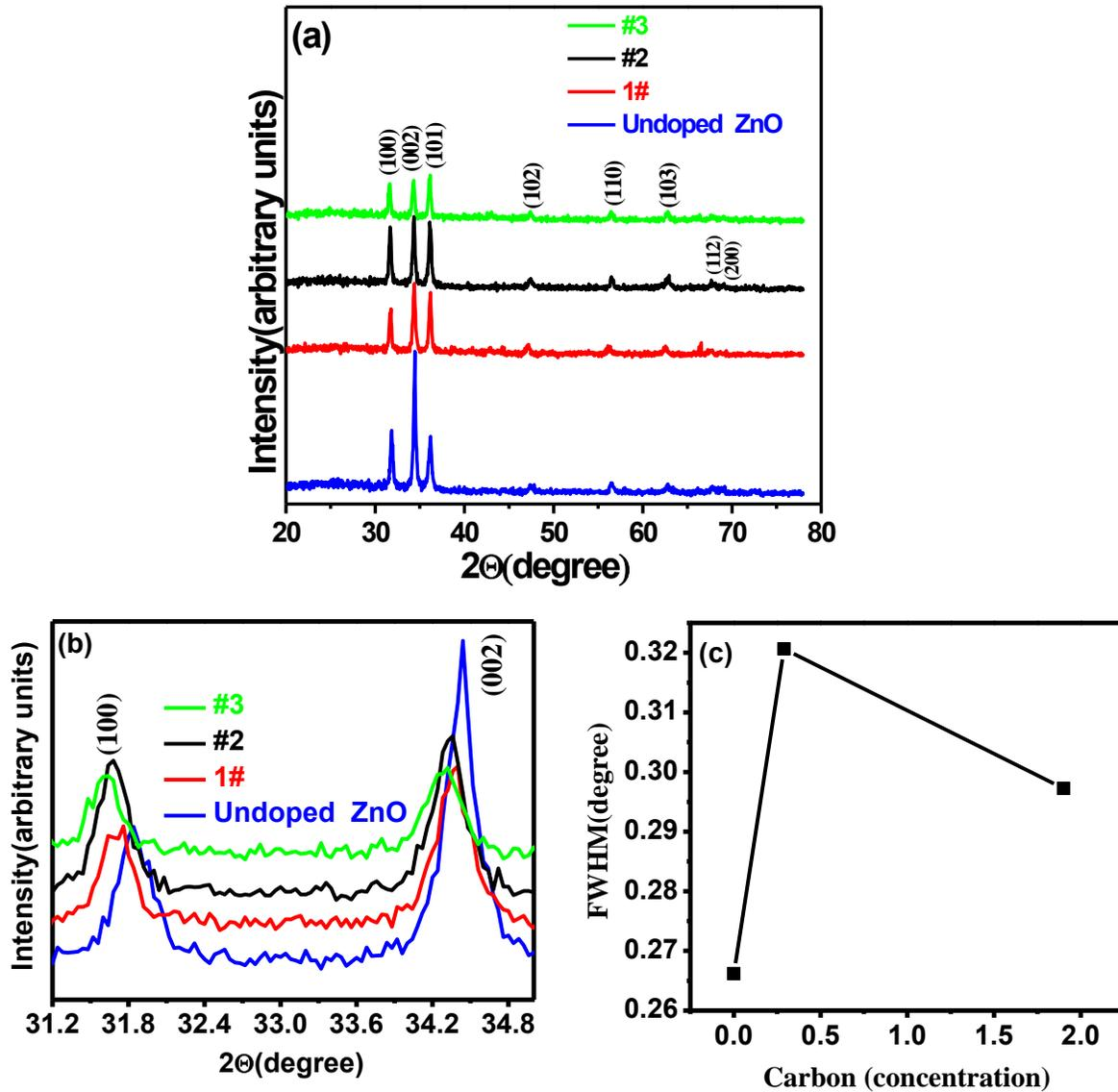
**Figure 3.1** (a) X-ray diffraction patterns of undoped and carbon-doped 300 nm thick ZnO films annealed at 500 °C. (b) The enlarged XRD patterns of undoped ZnO, #1, #2 and #3 C-doped ZnO samples. (c) Variation of full width half maximum (FWHM) values of the (002) peak with Carbon concentration.
