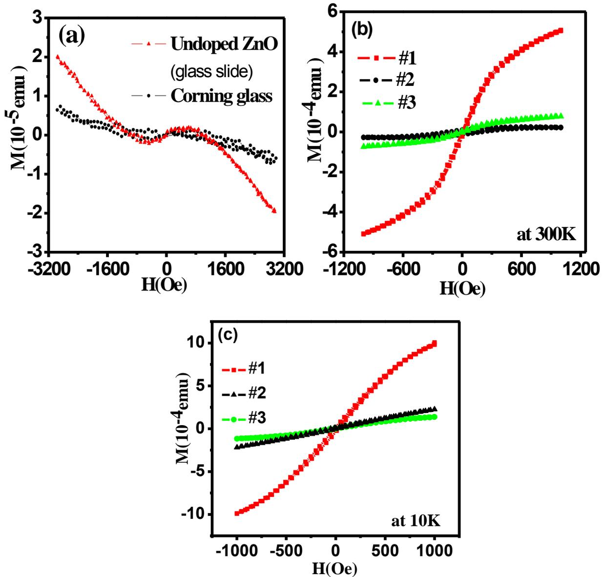
**Figure 3.4** Hysteresis loops for (a) Undoped ZnO (on glass slide) and Corning glass at room temperature and #1, #2 and #3 samples at (b) 300 K and (c) 10 K
