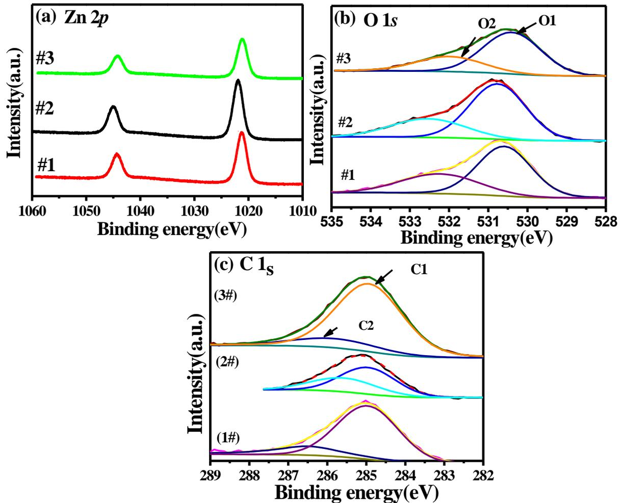
**Figure 3.3** XPS spectra of (a) Zn 2*p*, (b) O 1*s* and (c) C 1*s* core level regions of #1, #2 and (#3) samples. Data (black line) and fits (coloured line) are shown (for details see text).
