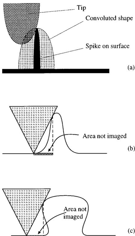
FIG. 1. Dilatation of tip and surface (a), resulting in loss of information on single (b) and not single (c), valued surfaces.
