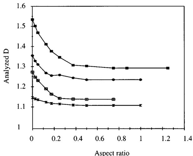
FIG. 3. The analyzed fractal dimension  $D$  from a simulated surface as a function of the aspect ratio of the tip. The intersection of the curves with the vertical axis gives the initial fractal dimension of the surface.
