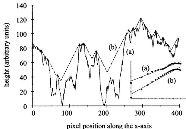
FIG. 2. Height profile of the fractal surface (a) before and (b) after dilation. The inset shows the one-dimensional correlation function analysis, plotting  $\log [S(\Delta x)]$  against  $\log (\Delta x)$ . This results in (a)  $D=1.51$  before dilation and (b)  $D=1.34$  after dilation.
