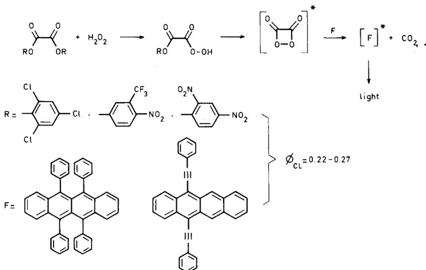
Fig. 3. Indirect chemiluminescence from oxalate ester oxidation
