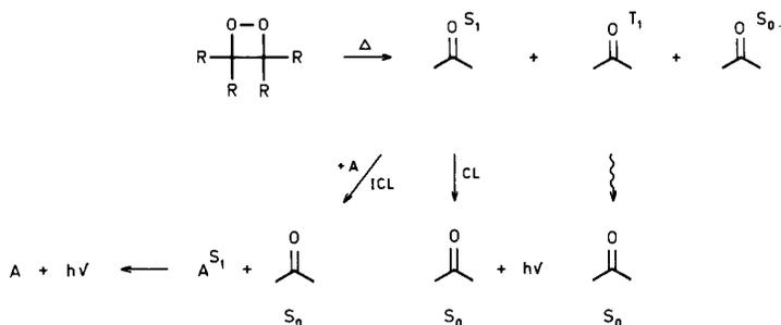
Fig. 5. Pathways for electronic energy in 1,2-dioxetane decomposition
