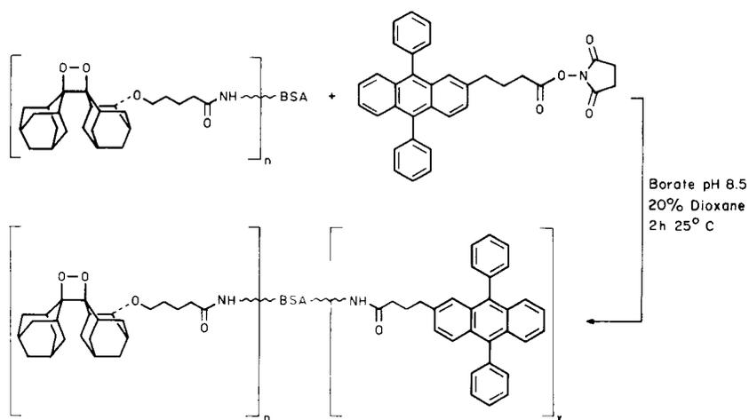
Fig. 12. Preparation of dual labelled BSA
