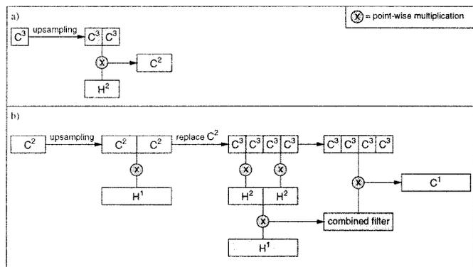
Fig. 7. (a) Computation of  $C^2$  from  $C^3$  via upsampling followed by multiplication. (b) Computation of  $C^1$  from  $C^3$  directly. The filters  $H^2$  and  $H^1$  are combined into a new filter, and  $C^3$  is upsampled twice. Multiplication yields  $C^1$ .
