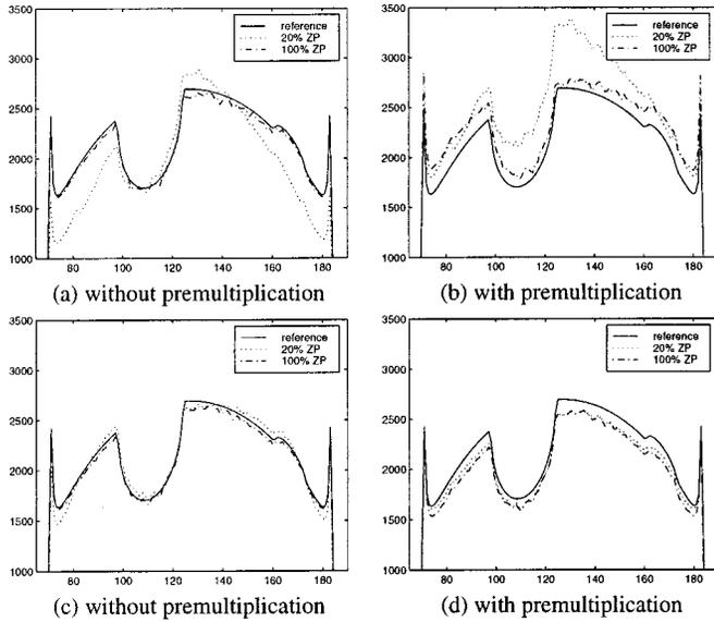
Fig. 4. Profiles of FVR renderings of the head phantom along the line  $x = 122$ . (a) and (b) linear interpolation, (c) and (d) cubic spline interpolation. The reference profiles are obtained by analytical computation.
