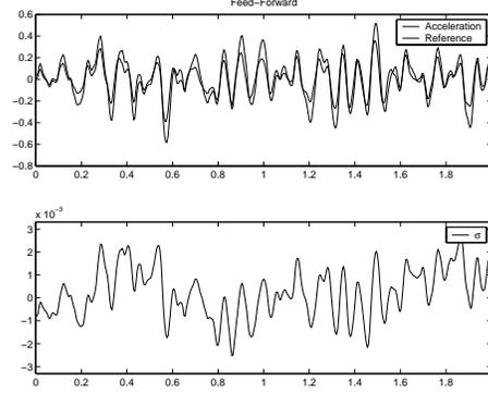
Fig. 2. Simulation results with feed-forward controller only.
