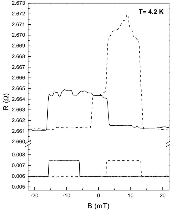
Figure 5.3: The spin valve effect of sample MSV2 in a conventional measurement geometry (top curve) at  $T = 4.2 \text{ K}$  and non-local measurement geometry (bottom curve), with a Py electrode spacing  $L = 250 \text{ nm}$ . The sizes of the Py electrodes are  $2 \times 0.8 \mu\text{m}^2$  (Py1) and  $14 \times 0.5 \mu\text{m}^2$  (Py2). The solid(dotted) curve corresponds with a negative (positive) sweep direction of the B-field.
