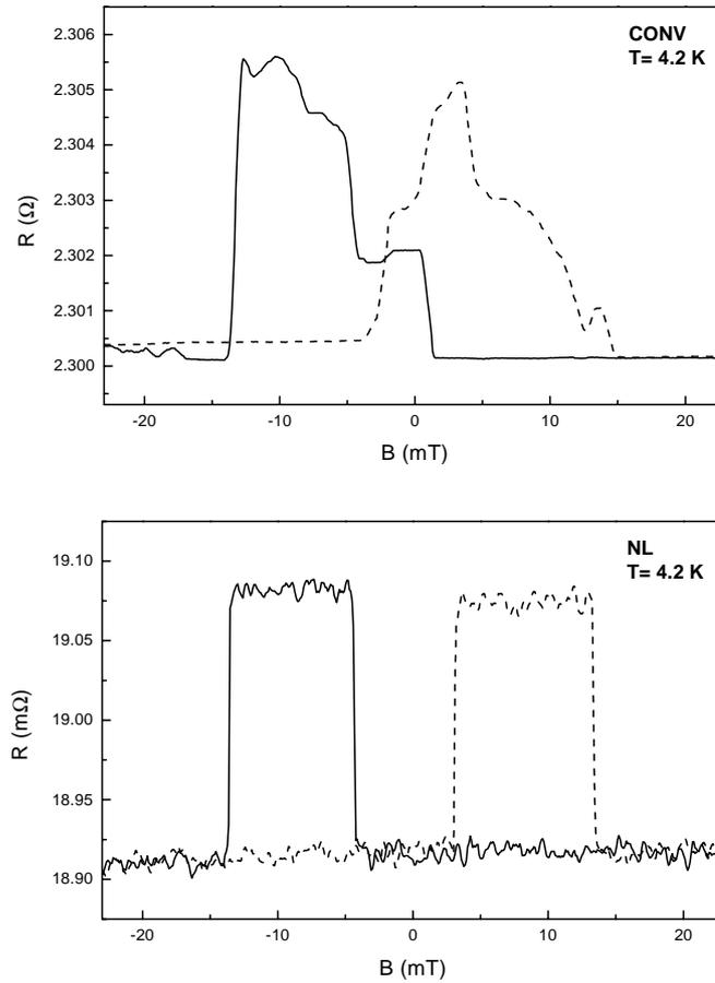
Figure 5.5: The spin valve effect of a Py/Al/Py sample using a conventional measurement geometry (CONV, top curve) at  $T = 4.2$  K and non-local measurement geometry (NL, bottom curve), with a Py electrode spacing  $L = 250$  nm. The sizes of the Py electrodes are  $2 \times 0.8 \mu\text{m}^2$  (Py1) and  $14 \times 0.5 \mu\text{m}^2$  (Py2). The solid (dotted) curve corresponds with a negative (positive) sweep direction of the B-field.
