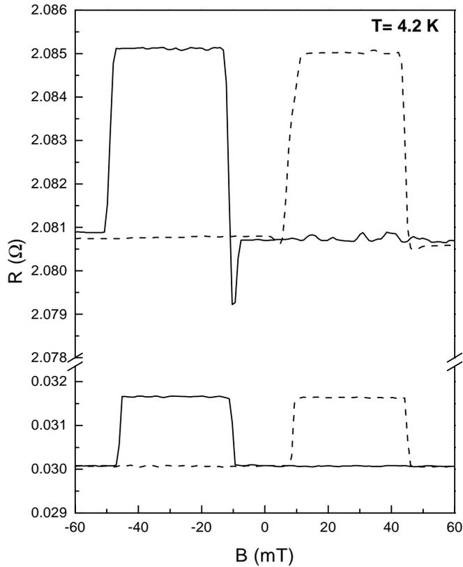
Figure 5.2: The spin valve effect of sample MSV1 in a conventional measurement geometry (top curve) at  $T = 4.2$  K and non-local measurement geometry (bottom curve), with a Py electrode spacing  $L = 250$  nm. The sizes of the Py electrodes are  $2 \times 0.5 \mu\text{m}^2$  (Py1) and  $14 \times 0.15 \mu\text{m}^2$  (Py2). The solid (dotted) curve corresponds with a negative (positive) sweep direction of the B-field.
