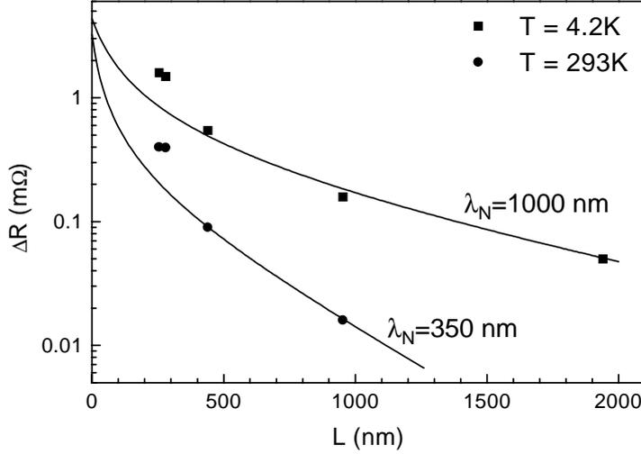
Figure 5.4: Dependence of the magnitude of the spin signal  $\Delta R$  on the Py electrode distance  $L$ , measured on Py/Cu/Py samples in the non local geometry. The solid squares represent data taken at  $T = 4.2$  K, the solid circles represent data taken at RT. The solid lines represent the best fits based on equation 2.31.
