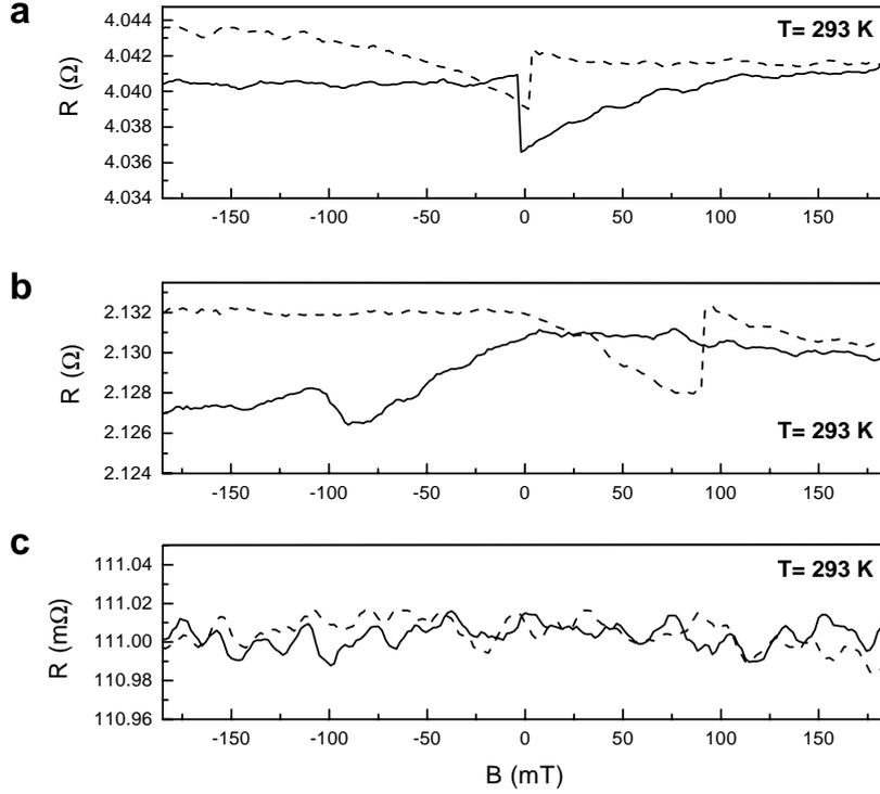
Figure 5.8: (a) "Contact" magnetoresistance trace (see text) of the Ni1 electrode with size  $2 \times 0.5 \mu\text{m}^2$ . (b) "Contact" magnetoresistance trace of the Ni2 electrode with size  $14 \times 0.15 \mu\text{m}^2$ . (c) The spin valve effect of a Ni/Cu/Ni device at RT with a Ni electrode spacing of  $L = 500 \text{ nm}$ , using a non local measurement geometry. The solid (dotted) curve corresponds with a negative (positive) sweep direction of the B-field.
