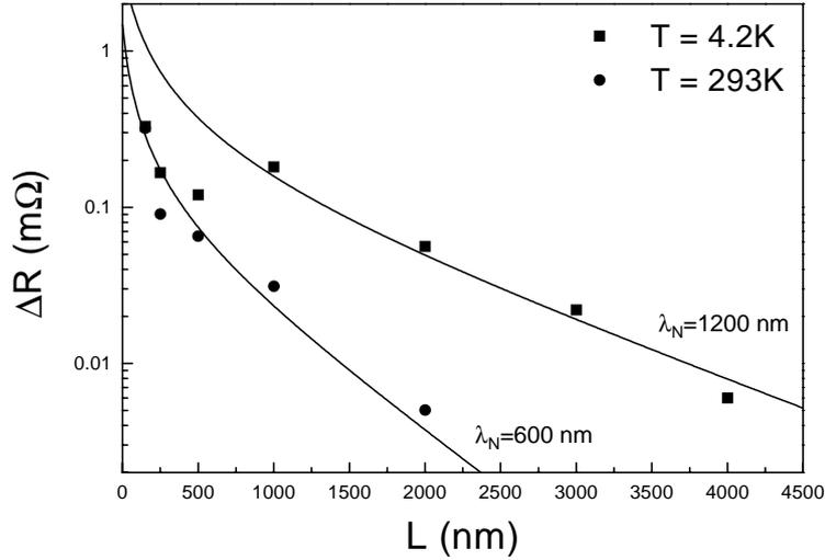
Figure 5.6: Dependence of the magnitude of the spin signal  $\Delta R$  on the Py electrode distance  $L$ , measured in the non local geometry for Py/Al/Py spin valves. The solid squares represent data taken at  $T = 4.2$  K, the solid circles represent data taken at RT. The solid lines represent the best fits based on Eq. 2.31.
