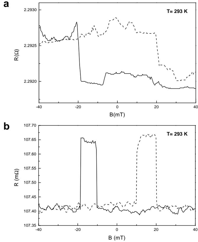
Figure 5.7: a, "Contact" magnetoresistance trace of the Co<sub>2</sub> electrode with size  $14 \times 0.5 \mu\text{m}^2$ . The Hall signal indicates an abrupt magnetization switching of the Co<sub>2</sub> electrode. b, The spin valve effect at RT in a Co/Cu/Co device with a Co electrode spacing  $L = 250 \text{ nm}$ , using the non local measurement geometry. The solid (dotted) curve corresponds with a negative (positive) sweep direction of the B-field.
