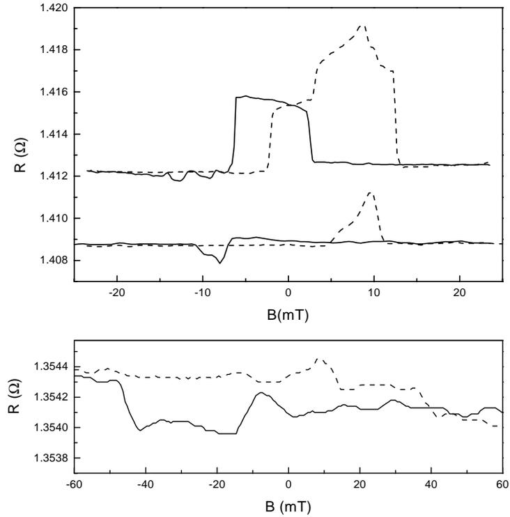
Figure 4.4: 'Contact' magnetoresistance behavior at  $T = 4.2$  K of the Py/Cu contact area for Py electrodes with dimensions  $2.0 \times 0.8 \mu\text{m}^2$  (top),  $2.0 \times 0.5 \mu\text{m}^2$  (middle) and  $14.0 \times 0.15 \mu\text{m}^2$  (bottom). The solid (dotted) curve corresponds with a negative (positive) sweep direction of the B-field, which is applied parallel to the long (easy) axis of the Py electrode.
