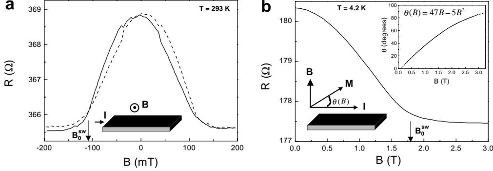
Figure 4.2: Perpendicular AMR of a  $0.2 \times 12 \mu\text{m}^2$  Co electrode, (a) with the magnetic field  $B$  applied perpendicular the Co strip but parallel to the substrate plane at RT and (b) with the magnetic field  $B$  applied perpendicular to the substrate plane at  $T = 4.2$  K. The inset in (b) shows the angle between the magnetization  $\mathbf{M}$  and the direction of the current through the wire, see text.
