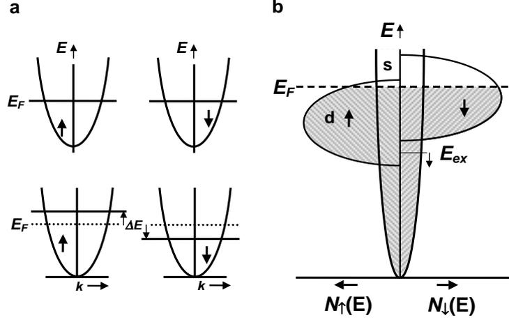
Figure 2.1: (a) Schematic illustration to derive the Stoner criterium of ferromagnetism, see text. (b) Band structure of a ferromagnetic metal in the simple Stoner picture. The d spin sub-bands are shifted in energy due to the exchange interaction, leading to a finite magnetization and a difference in the densities of states ( $N_{\uparrow}$ ,  $N_{\downarrow}$ ) and Fermi velocities at the Fermi-energy ( $E_F$ ).
