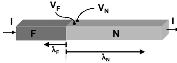
Figure 2.2: Schematic representation of the experimental layout for electrical spin injection. A current  $I$  is flowing through a F/N interface. The arrows indicated with  $\lambda_F$  and  $\lambda_N$  on either side of the F/N interface represent the distance where the spin accumulation exists in the F and N metal. The spin accumulation can be probed by attaching a F and N voltage probe to N within a distance  $\lambda_N$  from the F/N interface.
