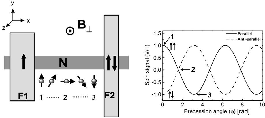
Figure 2.10: Oscillatory modulation of the spin valve signal ( $V/I$ ) in a ballistic nonmagnetic metal or semiconductor strip  $N$ . The label 1,2 and 3 refer to a precession angle of  $0$ ,  $90$  and  $180$  degrees.
