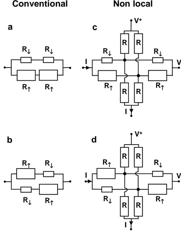
Figure 2.6: The equivalent resistor networks of the spin valve device. (a) The conventional spin valve geometry in parallel and (b) in anti-parallel configuration. (c) The non-local spin valve geometry in parallel and (d) in anti-parallel configuration.
