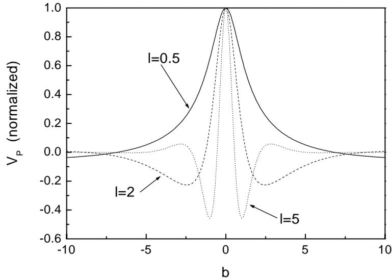
Figure 2.12: Precession signal.  $V_P$  is plotted as a function of the reduced magnetic field parameter  $b$  for several values of the reduced injector-detector separation  $l$  (see text for their definition)
