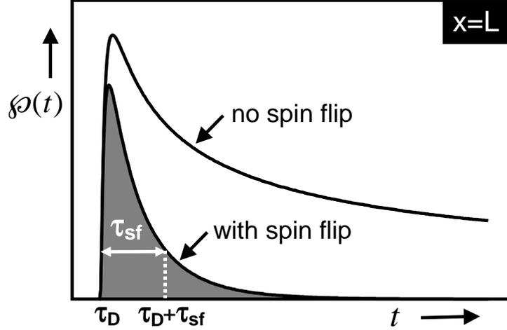
Figure 2.11: Probability per unit volume that, once an electron is injected, will be present at  $x = L$  without spin flip ( $\varphi(t)$ ) and with spin flip ( $\varphi(t) \cdot \exp(-t/\tau_{sf})$ ), as a function of the diffusion time  $t$ .
