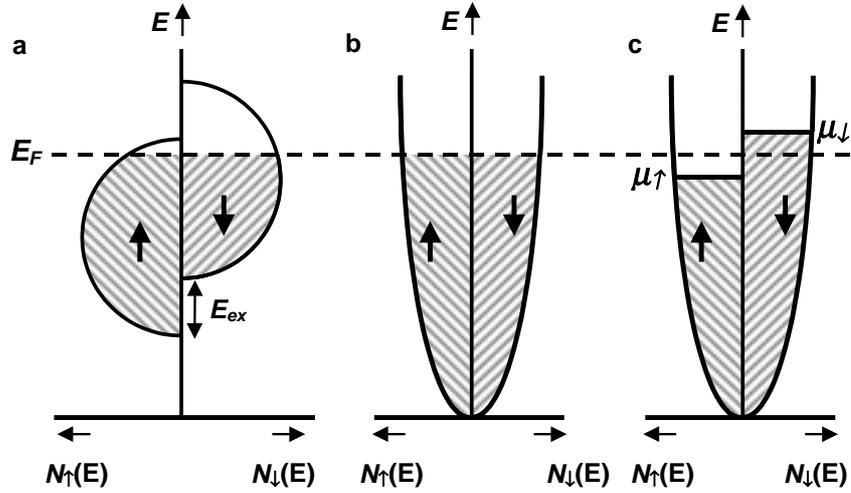
Figure 2.3: (a) Schematic representation of the spin dependent DOS and occupation of the  $d$  states in a ferromagnetic metal. (b) Unpolarized DOS of the free electron like  $s$  states in a nonmagnetic metal. (c) Spin accumulation in a nonmagnetic metal: the induced magnetization. The non-equilibrium population of the spin-up and spin-down states is caused by the injection of spin polarized current.
