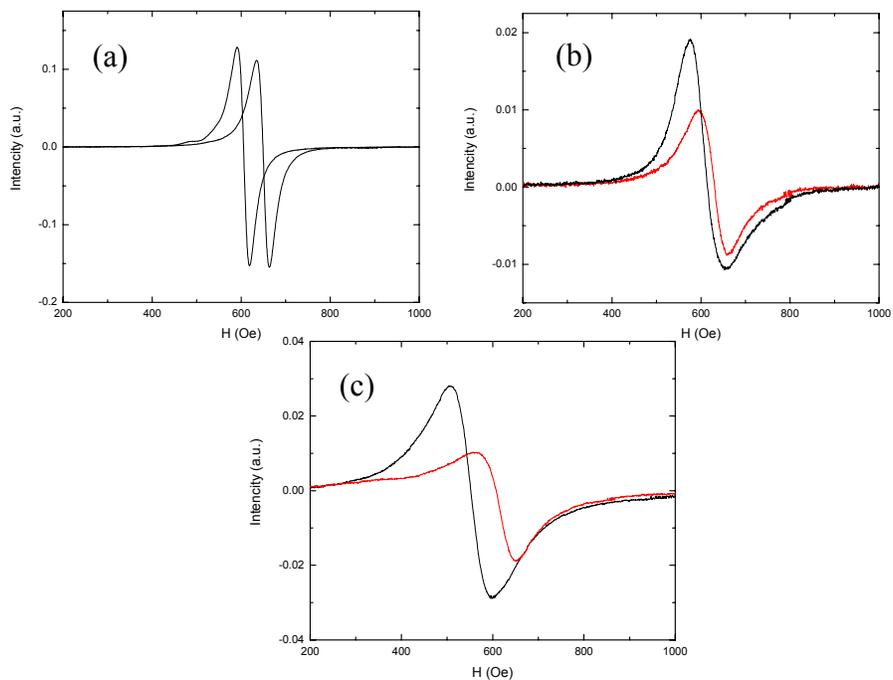
Fig. 5.4 ESR spectra of samples A – a, B – b and C – c measured with  $H_{DC}$  in the plane of the sample, parallel and perpendicular to the EA.
