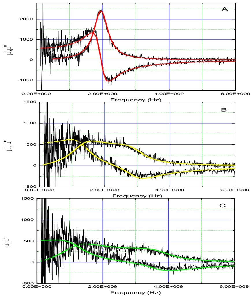
Fig. 5.6 Measurement and simulation of real and imaginary part of the complex permeability for sample A – (a), B – (b) and C – (c).
