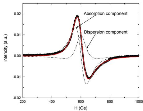
Fig. 5.5 ESR measurement for sample B: Experimental data is represented by circles, the absorption and dispersion components are indicated by arrows and the fit of the experimental data is represented by the continuous line.
