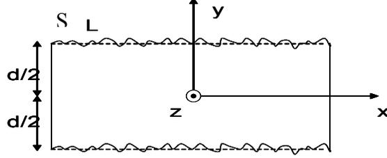
Fig. 5.2 The cross section of the film lying in the  $x$ - $z$  plane;  $d$  is the film thickness;  $S$  is the film boundary defined by  $d/2+h(x,z)$
