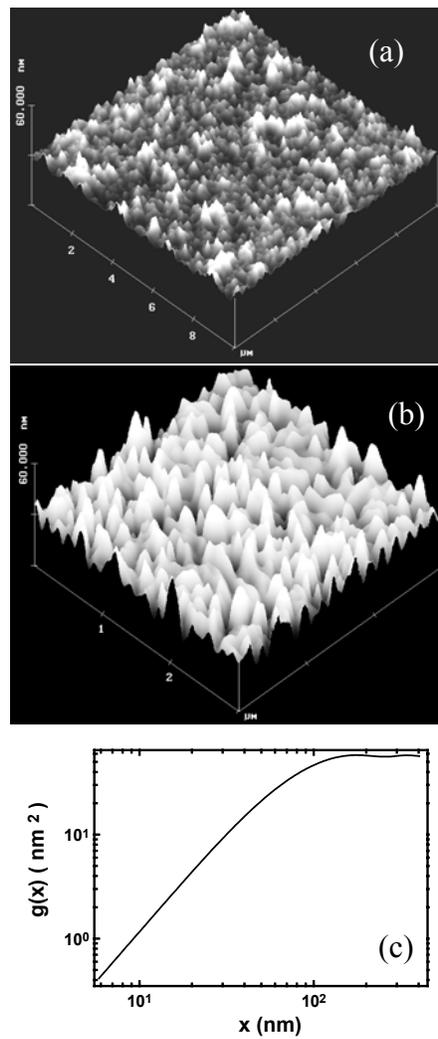
Fig. 5.1. AFM scans of the samples B (a) and C (b); height difference correlation function corresponding to sample C
