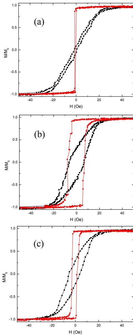
Fig. 5.3 Hysteresis loops of the samples A - a, B - b and C - c; measurements performed parallel and perpendicular to the easy axis.
