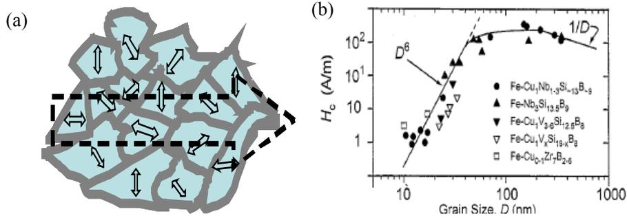
Fig. 1.3. a) Schematic representation of a nanocrystalline structure; left-right arrows indicate the orientation of the local easy axis and the dashed arrow indicates the average orientation of the magnetization. b) coercivity  $H_c$  versus average grain size [26]
