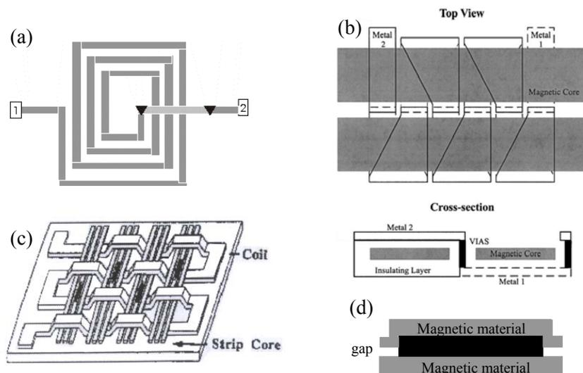
Fig. 1.1 Examples of high frequency inductors. a) spiral inductor, b) top view and cross-section of a planar inductor with two magnetic cores, c) thin film cloth-structured inductor with magnetic strip core array, d) geometry of the electromagnetic model for a magnetic sandwich inductor with variable edge gaps
