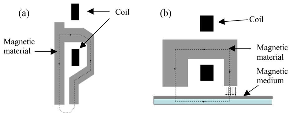
Fig. 1.2. Schematic drawings of a (a) longitudinal writing head and (b) perpendicular writing head and a magnetic medium with a soft underlayer.
