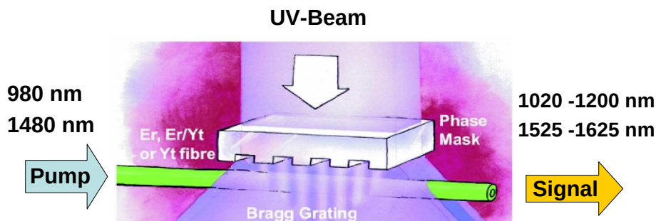
Figure 4.6: Principle and basic components of a DFB fiber laser [taken from KOHERAS brochure]. It consists of a fiber Bragg grating written in an actively doped fiber pumped at 980 nm or 1480 nm with a semiconductor laser.
