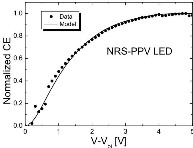
**Figure 6.4:** Normalized efficiency CE vs voltage for ITO/NRS-PPV/Ba/Al LED form experiment (●) and model (line). Exciton quenching parameters used are obtained in from optical experiments.
