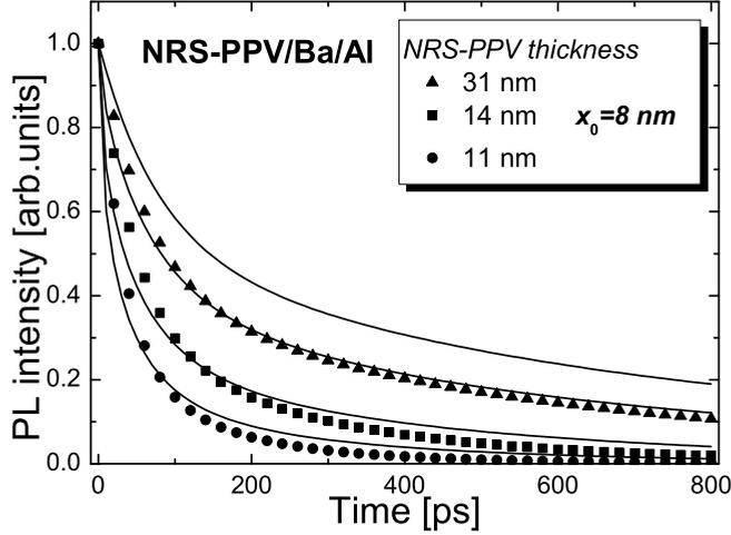
**Figure 6.1:** Deconvoluted and normalized PL decay curves in polymer/metal structures with variable polymer film thickness (symbols). Lines are fits of these data to Eq. (6.1) with  $x_0 = 8$  nm and  $D = 3 \times 10^{-4}$  cm<sup>2</sup>/s.
