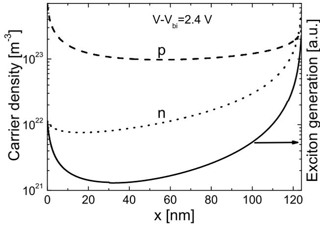
**Figure 6.2:** Hole ( $p$ , dashed curve) and electron ( $n$ , dotted curve) density distribution in the cross-section of the device simulated with a PLED model. Also shown is the exciton generation profile (solid curve) assuming Langevin recombination of the charge carriers.
