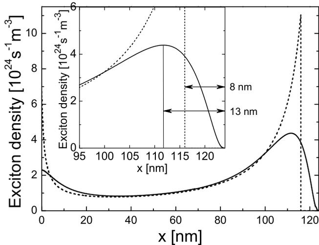
**Figure 6.3:** Exciton density profile (solid curve) simulated for a bias voltage of 2.4 V. Exciton profile (as implied in Ref. [6]) is shown for comparison (dashed curve).
