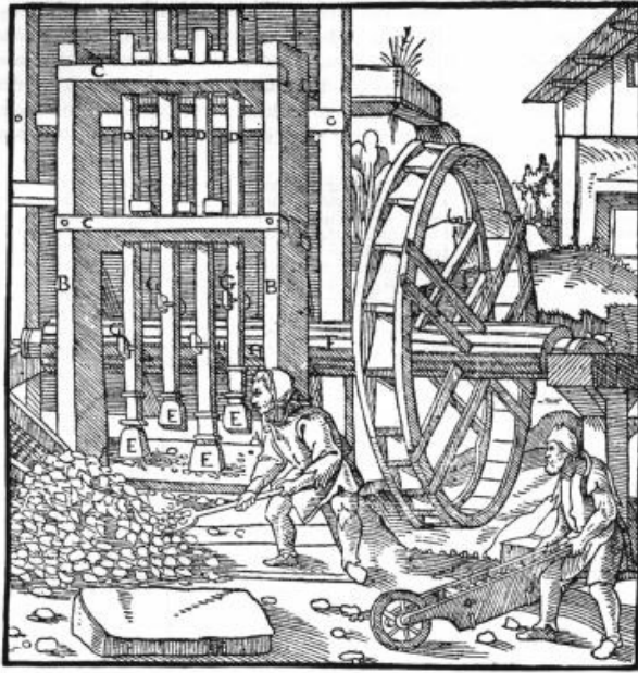
A—MORTAR. B—UPRIGHT POSTS. C—CROSS-BEAMS. D—STAMPS. E—THEIR HEADS. F—AXLE (CAM-SHAFT). G—TOOTH OF THE STAMP (TAPPET). H—TEETH OF AXLE (CAM).
