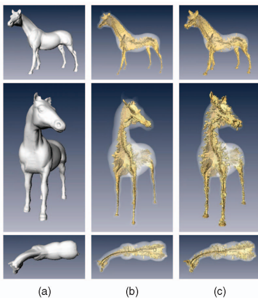
Fig. 5. Volume renderings of binary horse data ( 128 \times 280 \times 232 voxels) and its skeletons (side, front, and top views). First column: Input data. Second column: IMA-CP skeleton with \gamma = 7 . Third column: IMA-SRP skeleton. In the skeleton renderings, the input volume is rendered partially transparent.
