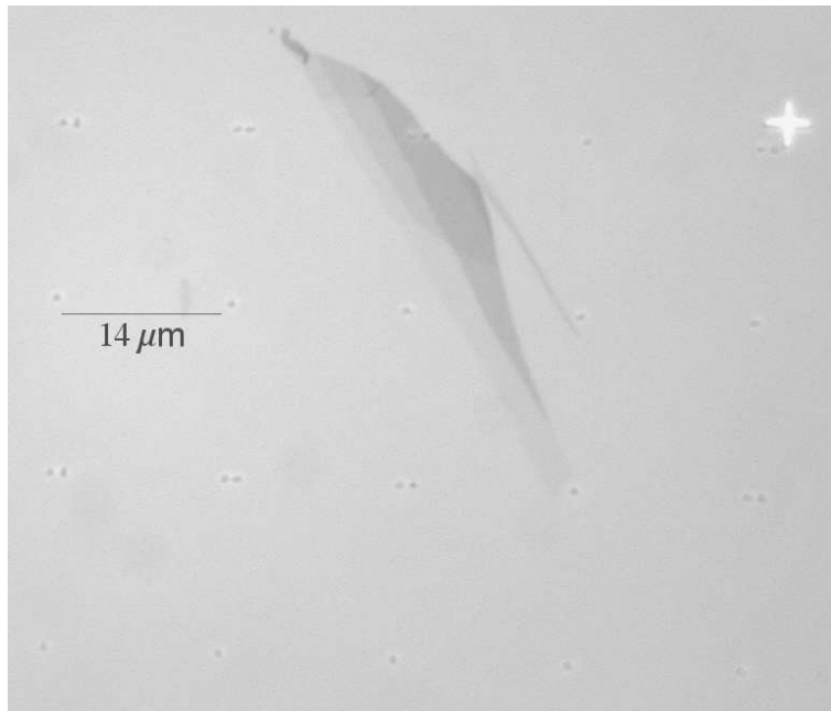
Figure 3.2: Optical image of a SiO 2 substrate covered with gold markers and a piece of HOPG graphite. The gold markers are separated by a distance of 14 μm. The position of the graphite layers with respect to the markers is known with a precision of 50 nm.
