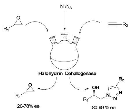
**Scheme 3** One-pot transformation from a racemic epoxide to an optically pure  $\beta$ -hydroxytriazoles
