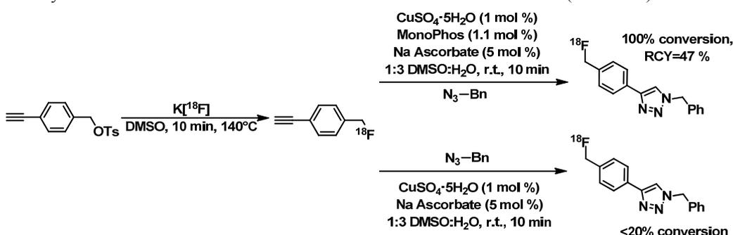
**Scheme 2** Demonstration of the acceleration of the CuAAC by MonoPhos
