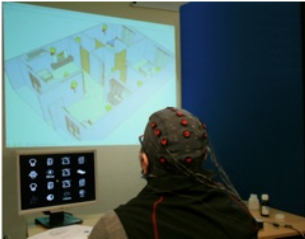
Fig. 2. BCI testing with active EEG electrodes g.GAMMAsys on the SM4All simulation environment.
