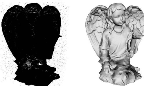
Fig. 11. Noise behavior. Left : noisy range data with 2 \cdot 10^6 samples and 4,000 outliers. Right : reconstructed surface, D = 10 . Angel data set courtesy of the U.C. Berkeley Computer Animation and Modeling Group.
