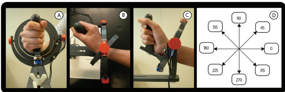
**Figure 6.1.** MR-compatible wrist device is shown with A) hand held in neutral position, B) wrist extension and C) radial deviation. D) Schematic overview of movement task consisting of 8 different out-of-centre movements. Out-of-centre stimuli appear randomly, and are always followed by a back-to-centre movement.
