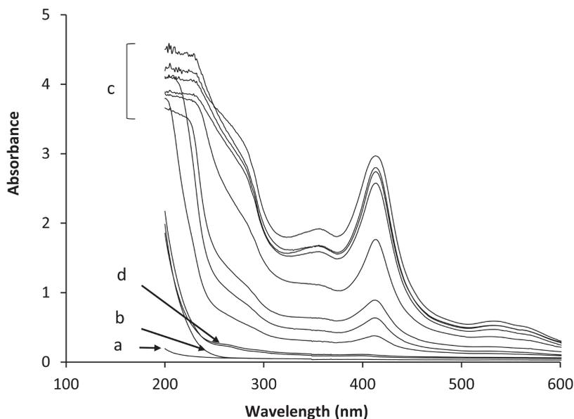
**Figure 1** UV-VIS absorbance of the precipitated DBS extracts using different EDTA concentrations. A: ACN: water (v/v 3:1); B: Blank extract using EDTA 1.54 g/L in water; C: Extracts of DBS using EDTA concentrations of 0–0.38 g/L in water; D: extracts of DBS using EDTA concentrations of 0.58–1.54 g/L in water.
