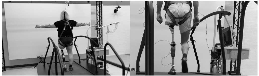
Figure 5. Treadmill test: the participant's movements are measured thanks to the reflective markers placed on their skin. The participant wore a harness for safety.
