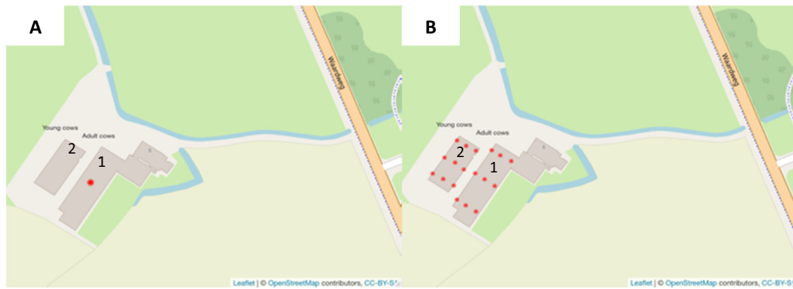
Fig. 3. Distribution of sources across barns (1) and (2), the red circle indicates the location of each individual source. (a) Single source. (b) Grid made of multiple sources, in this case, nine individual sources per each barn.
