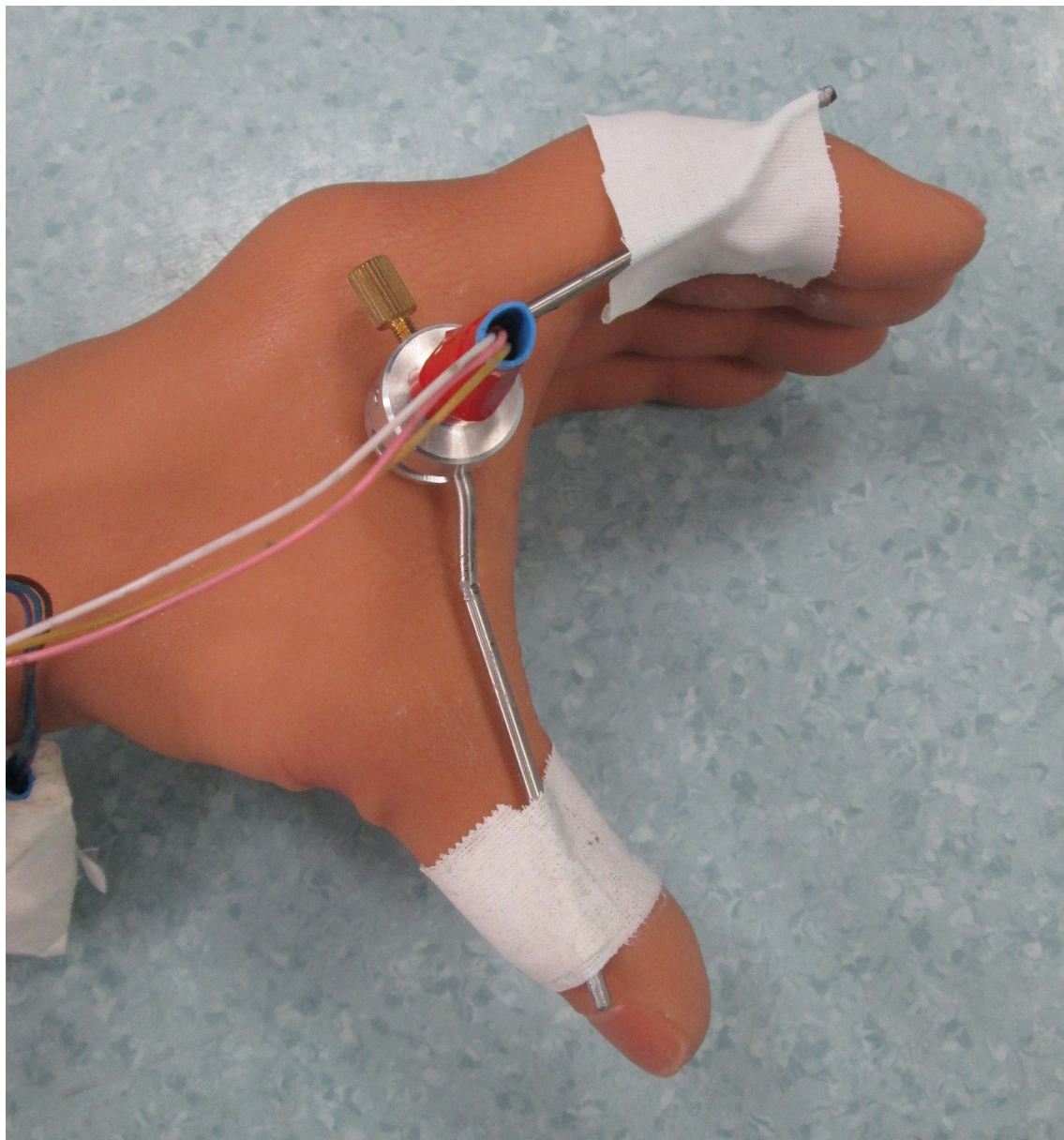
Fig 3. Potentiometer attached to the prosthesis hand.
