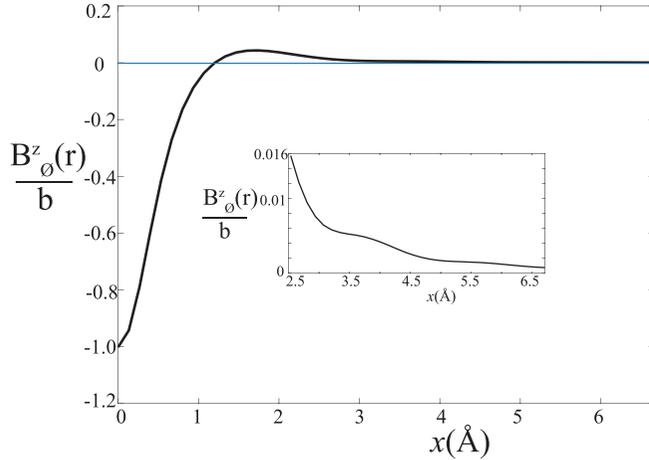
FIG. 3. The  $z$ -component of the Ørsted field near a RE atom in the free-electron gas.  $B_{\emptyset}^z = \mathbf{e}_z \cdot \mathbf{B}_{\emptyset}$ , as a function distance ( $\mathbf{r} = x\mathbf{e}_x$ ), where  $\mathbf{e}_j$  is the unit vector along the Cartesian axis  $j$ . The field is normalized by its modulus at the origin  $b = |\mathbf{B}_{\emptyset}(\mathbf{0})|$ .
