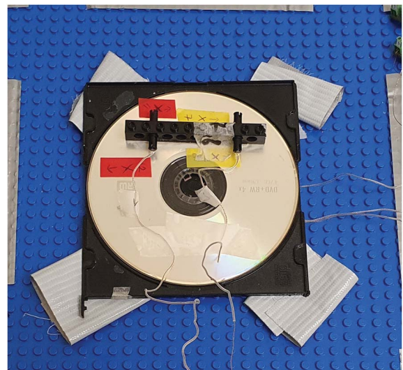
Figure 8. Sensors placed on CD (here depicted on the LEGO plate for easier visibility).
