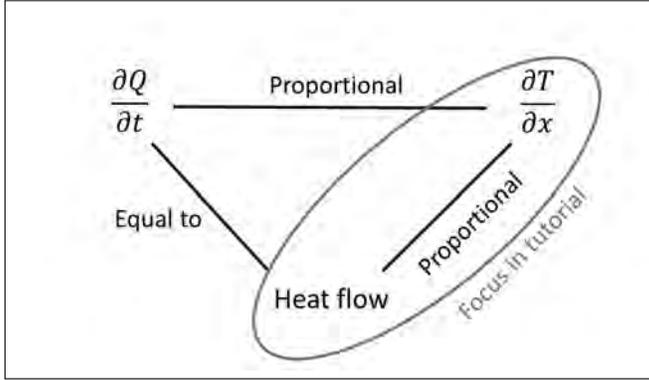
Figure 5.15: Visualization of the relation between heat flow and its descriptions in terms of time and position.
