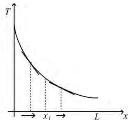
Figure 1.1: Graphical representation of a temperature distribution  $T(x)$  at a certain time  $t$ . The arrows visualize the heat flow through points nearby  $x_1$  (direction and strength).
