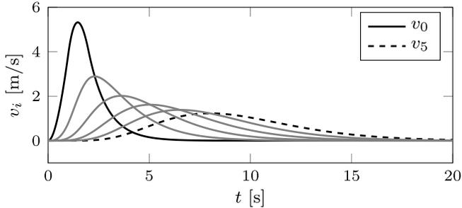
**Fig. 5.** Simulation of a platoon of six vehicles with time constants  $\tau_i$ ,  $i \in \{0, \dots, 5\}$  chosen randomly from the interval  $[0.6, 1.4]$ , time headway  $h = 1.5$ ,  $\gamma_i$  chosen randomly from  $[-0.1, 0.1]$ , and equilibrium initial conditions with  $x_i(0) = 0$ ,  $i \in \{1, \dots, 5\}$ . The input to the lead vehicle is given as  $u_0(t) = 10$  for  $t \in [0, 1]$ ,  $u_0(t) = -10$  for  $t \in [1, 2]$ , and  $u_0(t) = 0$  otherwise.
