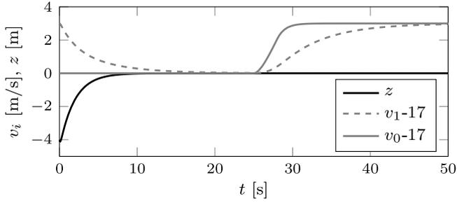
**Fig. 3.** Simulation of the two-vehicle model (7) for  $i = 1$ , time constants  $\tau_i$ ,  $i \in \{0, 1\}$  chosen randomly from the interval  $[0.6, 1.4]$ , time headway  $h = 1.5$ ,  $\gamma_1 = 0.1$ , and initial conditions  $x^T(0) = [-100 \ 20 \ 0 \ 0 \ 17 \ 0]$ . The input to the lead vehicle is given as  $u_0(t) = 1$  when  $t \in [25, 28]$  and  $u_0(t) = 0$  otherwise.
