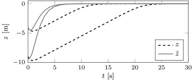
**Fig. 4.** A simulation of the spacing error  $z$  and  $\tilde{z}$  with different initial conditions. The error  $z$  is stabilized with the function  $\phi_2(z, \dot{z}) = -\tanh(z) - 2 \sinh(\dot{z})$ , whereas  $\tilde{z}$  is stabilized with  $\hat{\phi}_2(z, \dot{z}) = -z - 2\dot{z}$ .
